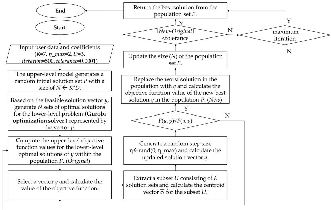
Figure 2. Solution steps flowchart for the hybrid algorithm in bi-level problem solving.
