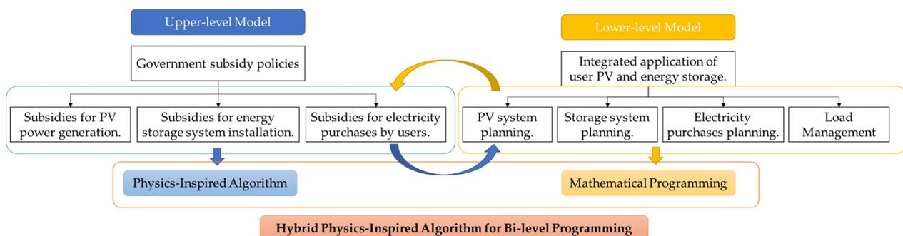
**Figure 1.** Framework diagram for bi-level problem of integrated PV and energy storage.
