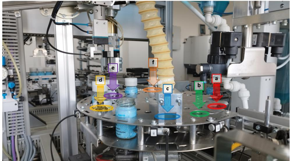
**Figure 5.** Filling Station of AFB Factory—(a) bottle entry; (b) liquid filling; (c) granulate filling; (d) cap placing; (e) cap closing; (f) bottle exit.
