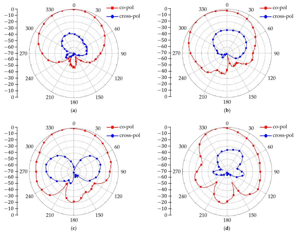
**Figure 28.** The measured E-plane radiation patterns of the proposed antenna: (a) At 3 GHz; (b) at 4 GHz; (c) at 5 GHz; (d) at 6 GHz.
