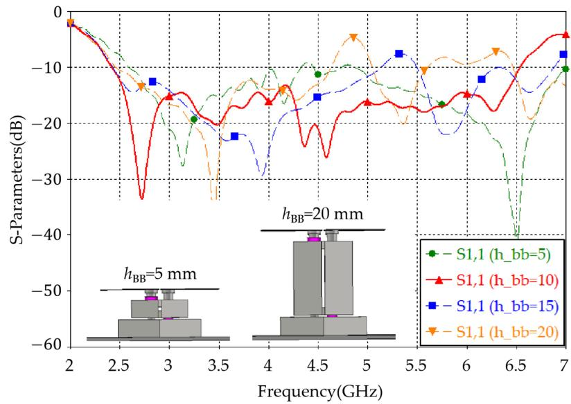
**Figure 14.** The relation between  $h_{BB}$  and the reflection coefficient  $S_{11}$ .
