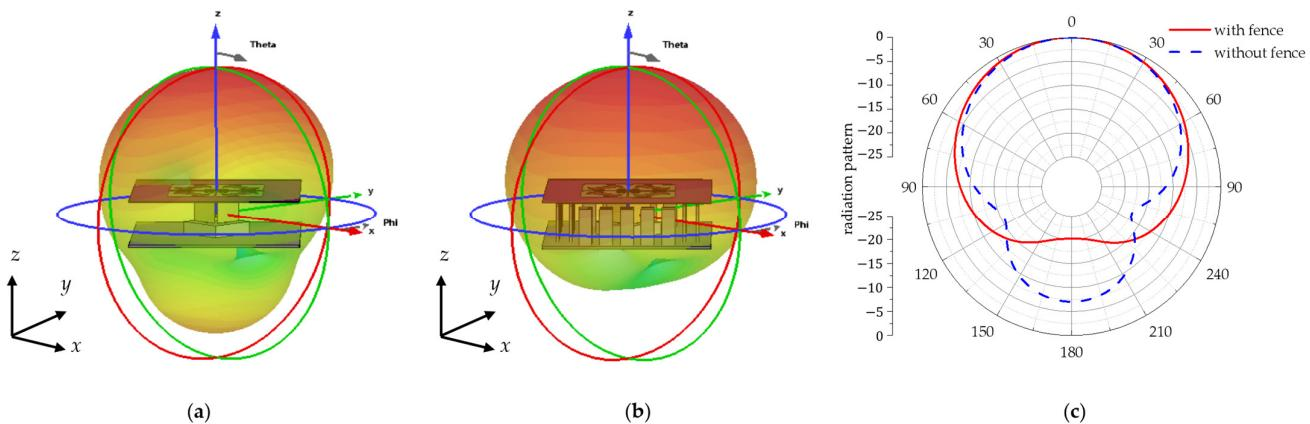
**Figure 22.** The 3D and 2D radiation patterns: (a) the 3D radiation pattern of the antenna model without the fences; (b) the 3D radiation pattern of the antenna model with fences; (c) the 2D radiation patterns of (a,b).
