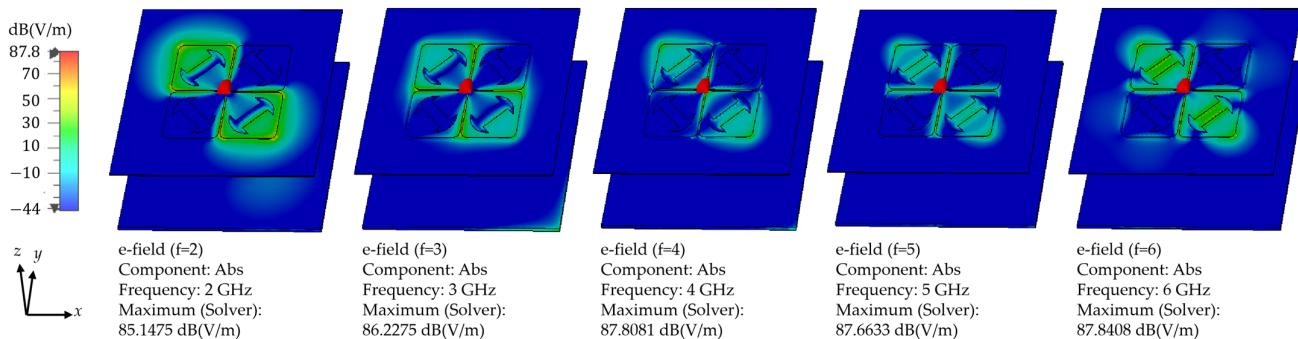
**Figure 20.** The absolute values of the electric field of the dipole antenna with HSVs.
