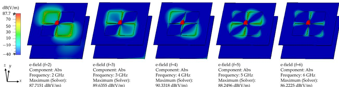
**Figure 18.** The absolute values of the electric field of the dipole antenna with SVs.
