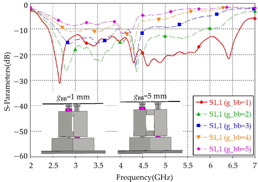
**Figure 16.** The relation between  $g_{BB}$  and the reflection coefficient  $S_{11}$ .
