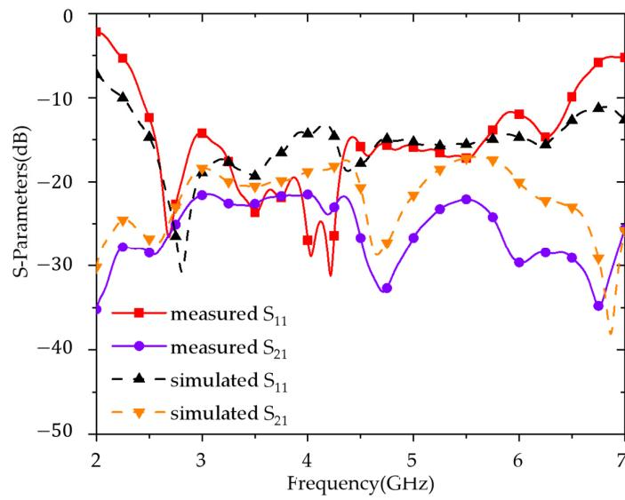
**Figure 25.** The simulated and measured  $S_{11}$  and  $S_{21}$ .
