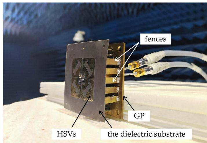
**Figure 26.** The setup for the radiation characteristics measurement.
