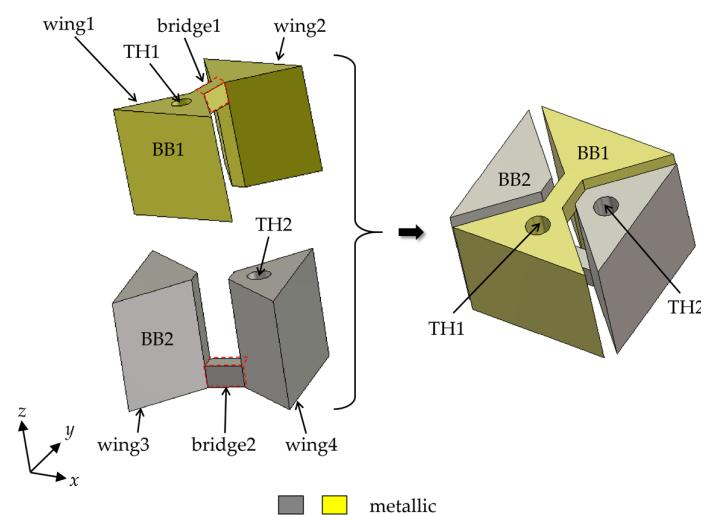
**Figure 6.** The installation of the two bow-tie baluns.
