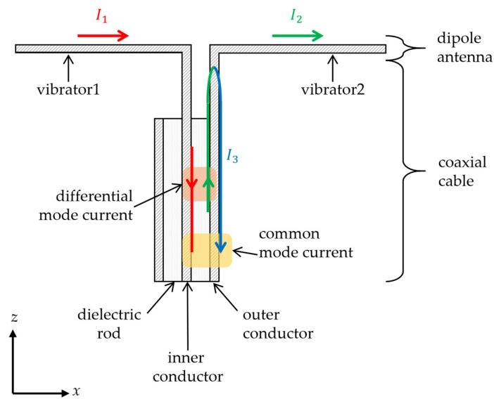
**Figure 1.** A dipole antenna fed by a coaxial cable.
