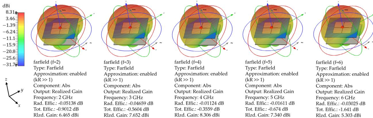
**Figure 19.** The 3-D radiation patterns of the electric field of the dipole antenna with SVs.
