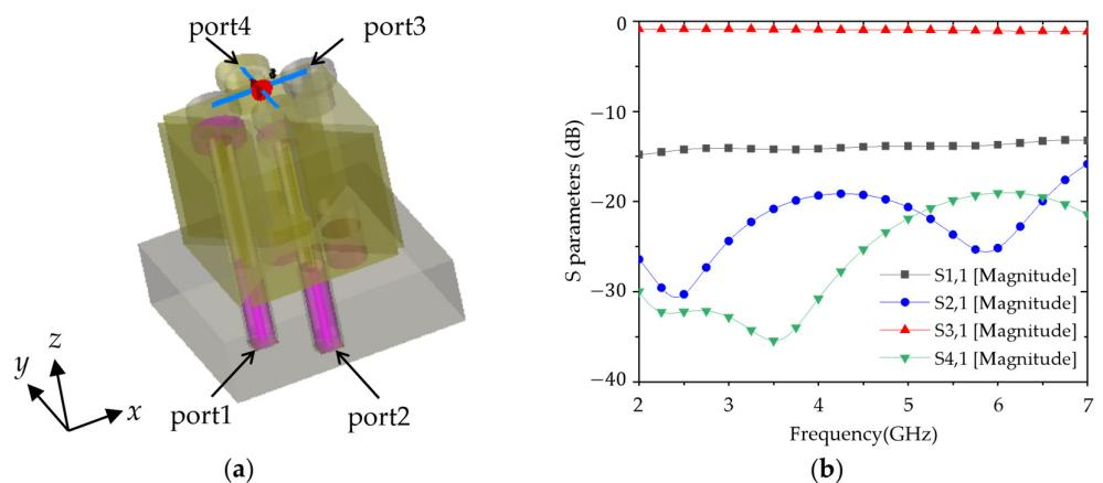
**Figure 13.** The S parameters of four ports: (a) The simulated model; (b) The simulated results of the S parameters of the four ports.
