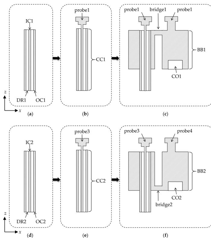
**Figure 2.** The evolution of the feed structure: (a) CC1; (b) IC1 loaded with probe1; (c) OC1 loaded with BB1; (d) CC2; (e) IC2 loaded with probe3; (f) OC2 loaded with BB2.
