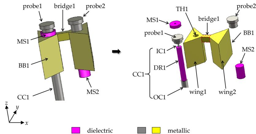
**Figure 5.** Explosion view of the feed structure for VPP.
