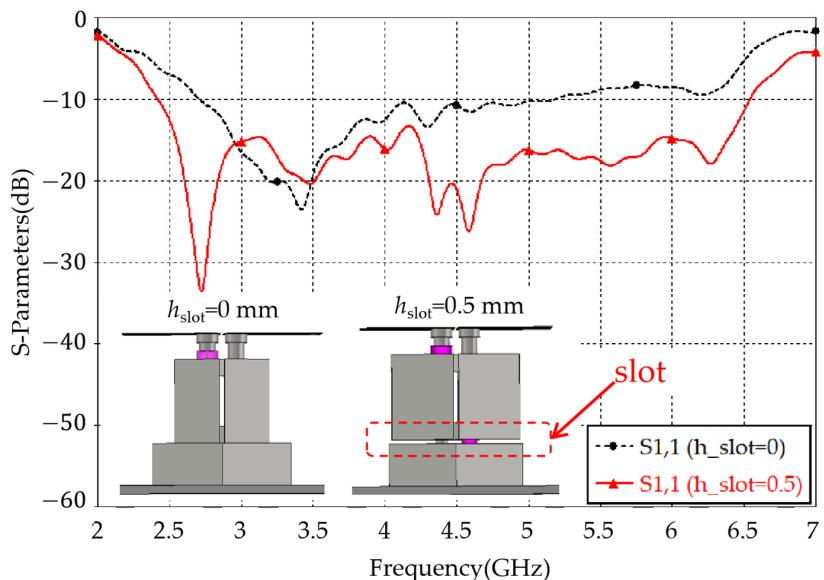
**Figure 17.** The relation between  $h_{slot}$  and the reflection coefficient  $S_{11}$ .
