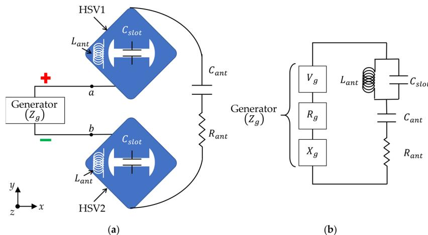
**Figure 8.** The dipole antenna loaded with H-shaped slots and its ECM: (a) The dipole antenna with HSVs; (b) the ECM of the dipole antenna with HSVs.
