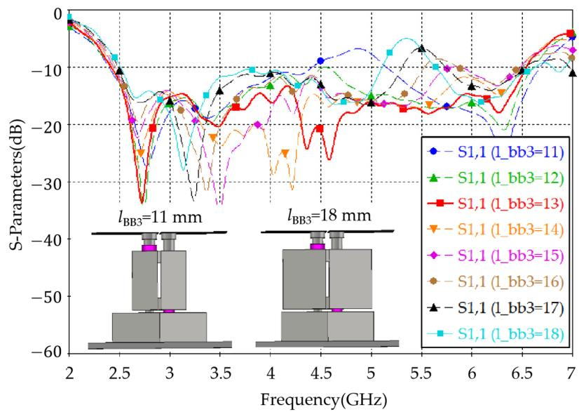
**Figure 15.** The relation between  $l_{BB3}$  and the reflection coefficient  $S_{11}$ .
