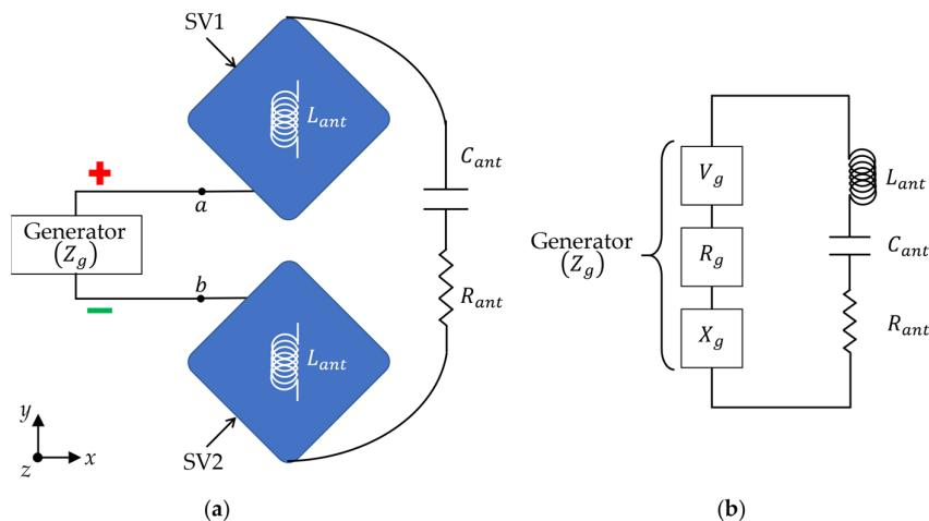
**Figure 7.** The regular dipole antenna with two square vibrators and its ECM: (a) The dipole antenna with SVs; (b) the ECM of the dipole antenna with SVs.
