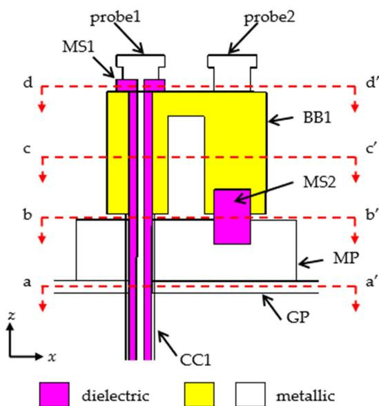
**Figure 9.** The cutting plane along the xoz plane. The red dashed lines (a-a', b-b', c-c', and d-d') represent the locations of the cutting planes along the xoy plane.
