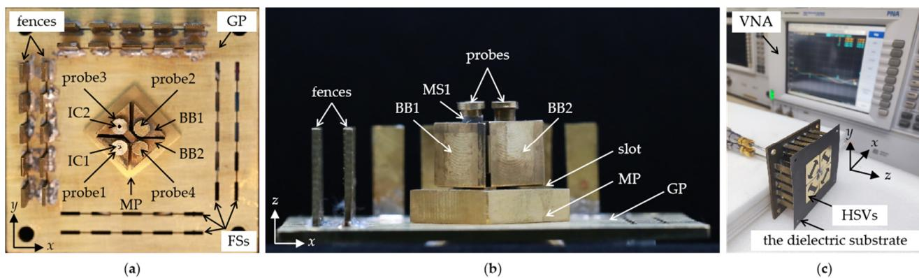
**Figure 24.** Photographs of the dipole antenna with HSVs and the test setup for  $S_{11}$ : (a) The top view; (b) the side view; (c) the test setup for  $S_{11}$ .
