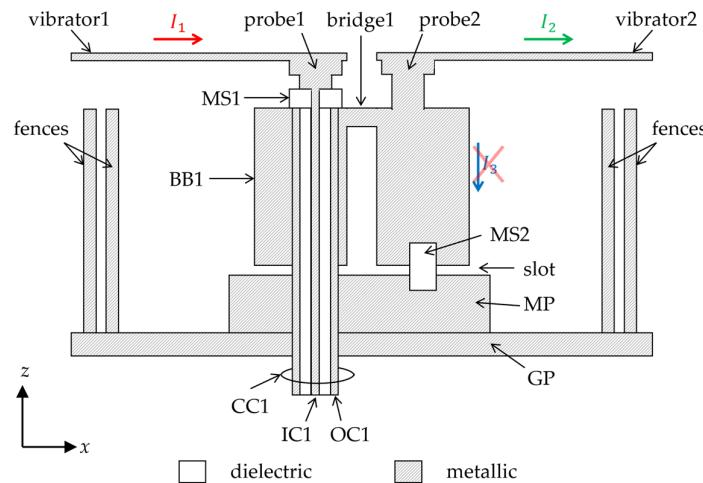
**Figure 3.** Schematic of the whole antenna structure for vertical polarization.
