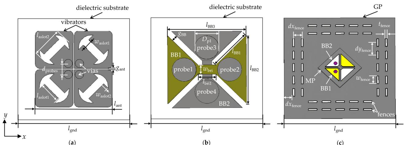
**Figure 12.** The dimensional parameters according to the cutting planes along the xoy plane: (a) The dimensional parameters of the antenna layer; (b) The dimensional parameters of the bow-tie balun; (c) The dimensional parameters of the ground plate and fences.
