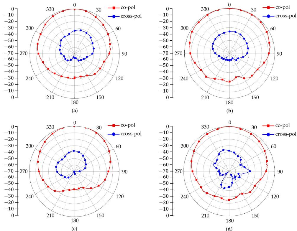
**Figure 29.** The measured H-plane radiation patterns of the proposed antenna: (a) At 3 GHz; (b) at 4 GHz; (c) at 5 GHz; (d) at 6 GHz.
