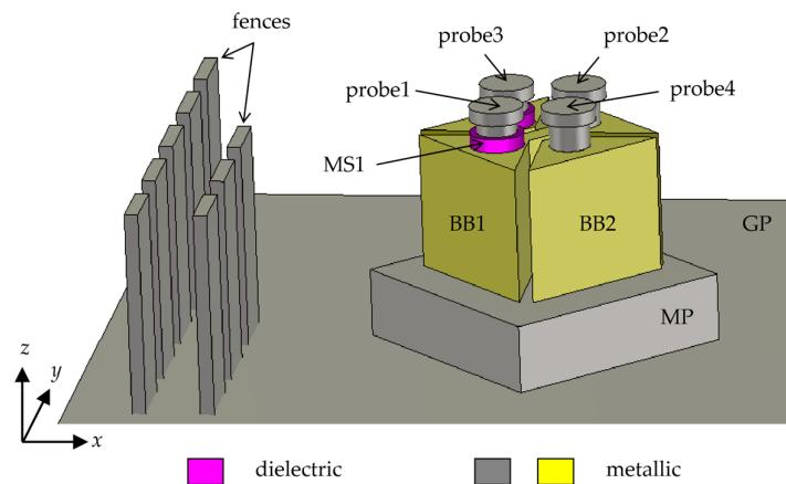
**Figure 4.** A 3D view of the proposed feed structure and ground reflector.
