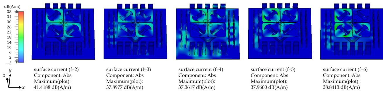
**Figure 23.** The surface current of the dipole antenna with HSVs.
