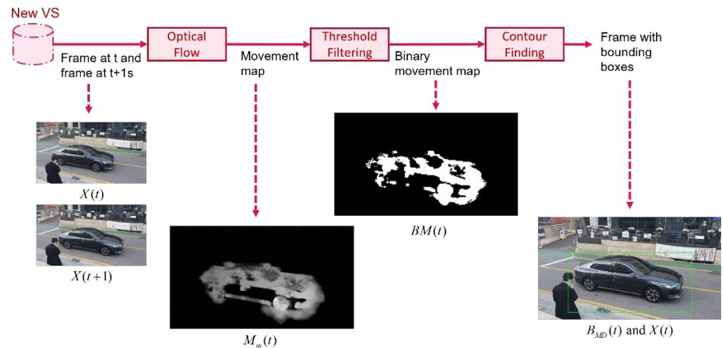
**Figure 2.** Steps of motion detector on filtering the frame from the target VS.
