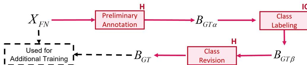
**Figure 3.** Interactive labeling process flow. Preliminary annotation and class revision is conducted by human (H) while class labeling is conducted by image classifier (IC), a ResNet18 model.
