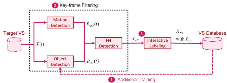
**Figure 1.** Overall diagram of key-frame extraction: (1) Additional training to improve the deep learning-based object detection model using data on the VS database, (2) key-frame filtering to collect the frames containing false negatives, and (3) interactive labeling for data annotation with less human effort.
