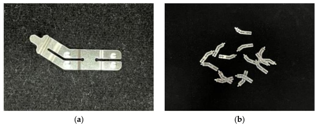
**Figure 8.** Appearance of nickel sheets. (a) Single nickel sheet; (b) Overlapping nickel sheets.
