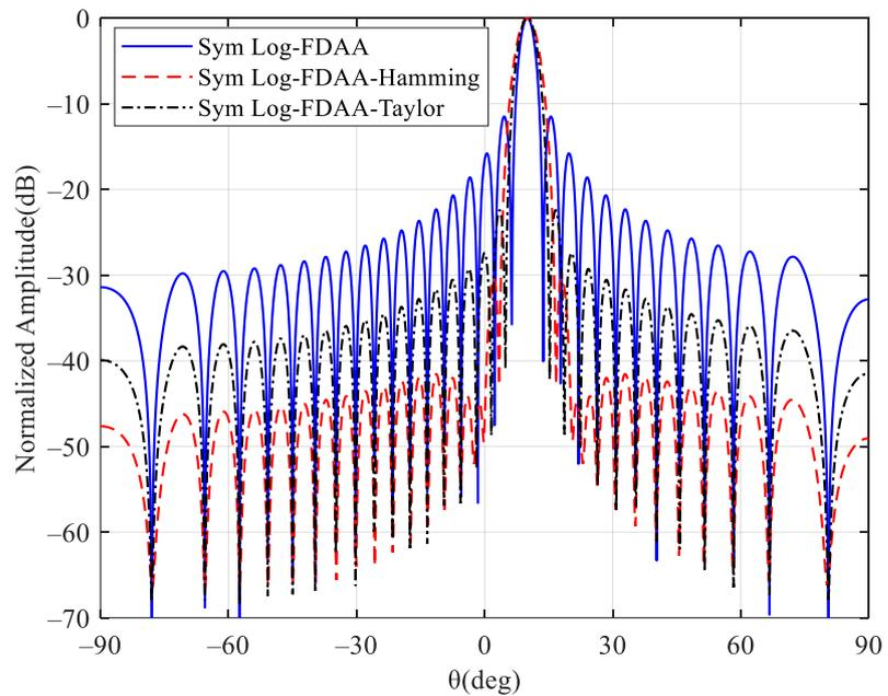
Figure 14. Comparison of beam pattern in angle dimension before and after optimization.
