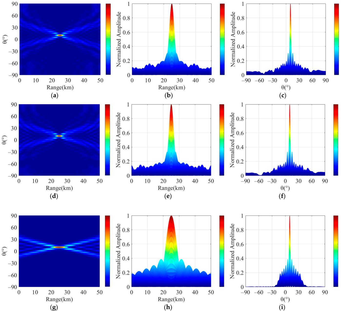
**Figure 11.** Beampattern synthesis results before optimization. (a) Sym Log-FDA. (b) Sym Log-FDA in the range domain. (c) Sym Log-FDA in the angle domain. (d) Sym Log-FDAA. (e) Sym Log-FDAA in the range domain. (f) Sym Log-FDAA in the angle domain. (g) Sym Hamming-FDAA. (h) Sym Hamming-FDAA in the range domain. (i) Sym Hamming-FDAA in the angle domain.
