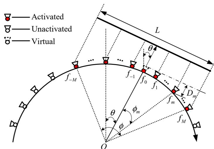
Figure 6. Phase compensation diagram of FDAA based on virtual the element.
