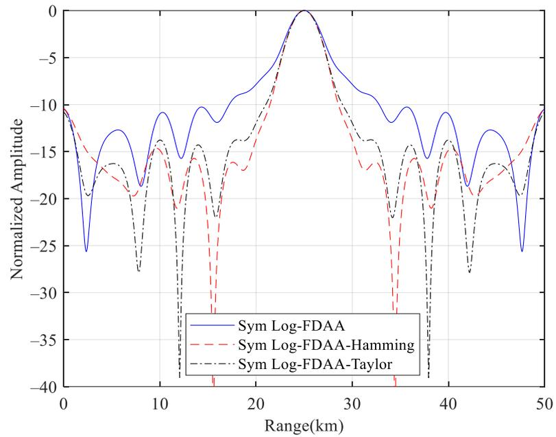
Figure 13. Comparison of beam pattern in range dimension before and after optimization.
