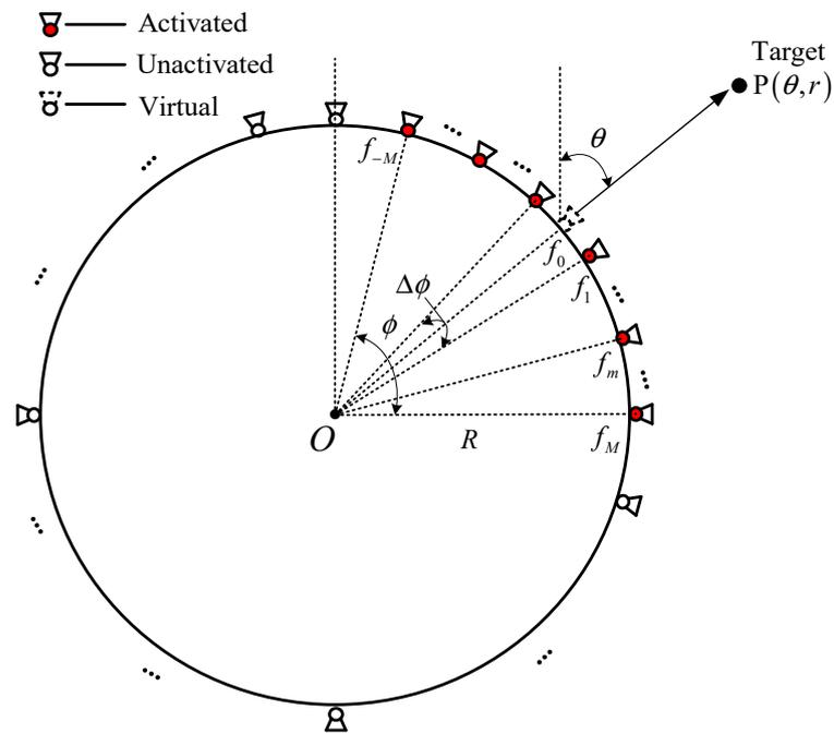
Figure 4. Beam scanning based on virtual element.
