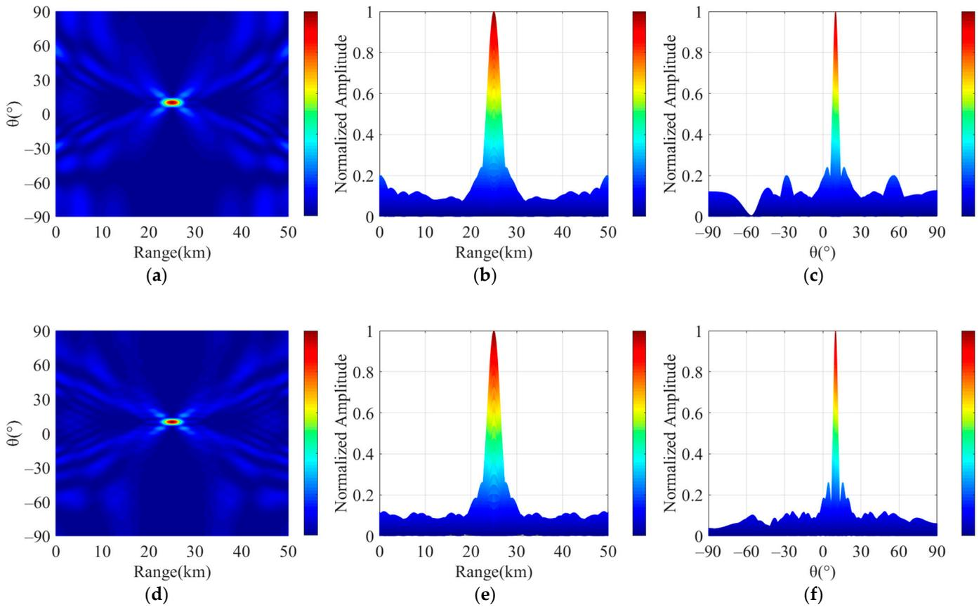
**Figure 12.** Beampattern synthesis results after optimization. (a) Hamming weighted Sym Log-FDAA. (b) Hamming weighted Sym Log-FDAA in the range domain. (c) Hamming weighted Sym Log-FDAA in the angle domain. (d) Taylor weighted Sym Log-FDAA. (e) Taylor weighted Sym Log-FDAA in the range domain. (f) Taylor weighted Sym Log-FDAA in the angle domain.
