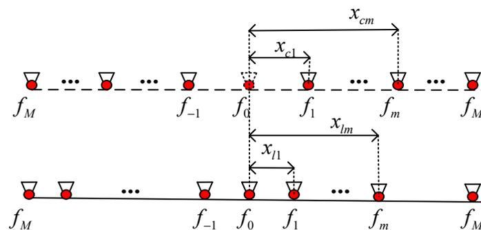
Figure 7. Comparison of equiphase plane based on virtual element and traditional FDA.
