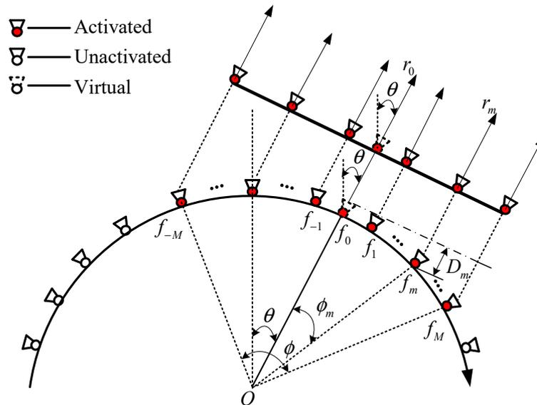
Figure 8. FDAA beampattern synthesis diagram based on virtual element.
