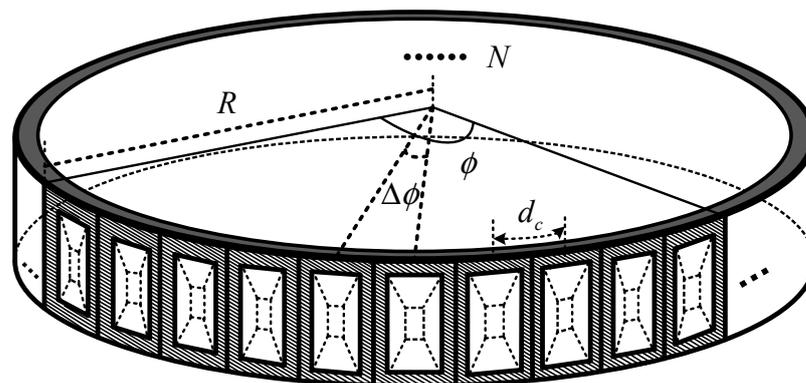
Figure 1. Three-dimensional geometric structure of FDAA.
