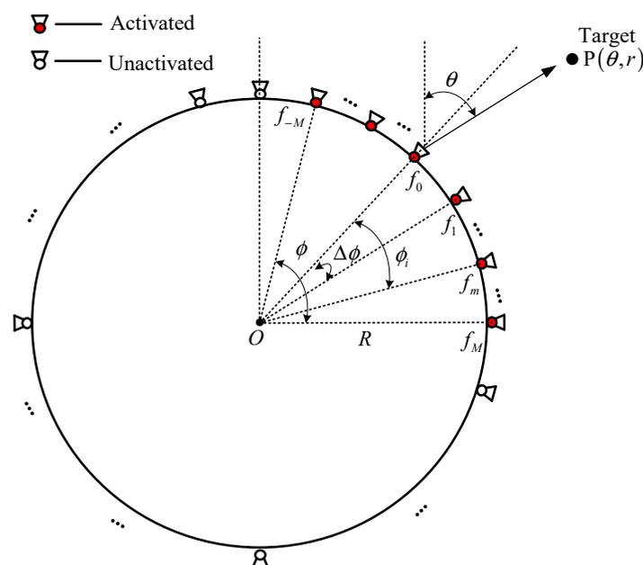
Figure 2. Two-dimensional geometric structure of FDAA.
