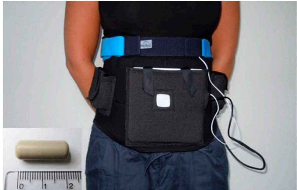
**Figure 2.** WIC, sensor array and receiver system presented by Motilis Medica when moving to an AC magnetic localization method [50] from their previous approach of using a permanent magnet within the WIC.
