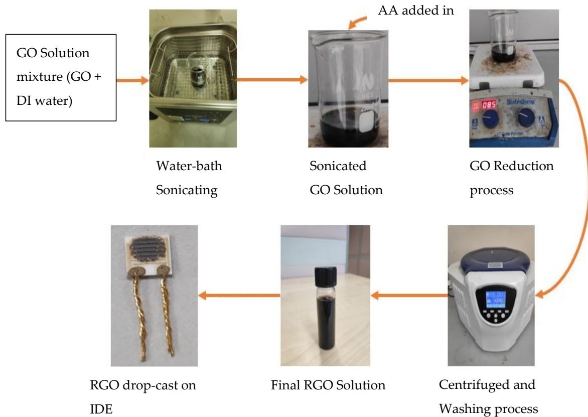
Figure 4. Illustration of RGO Preparation process from GO.
