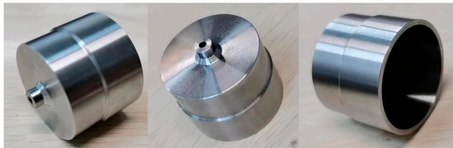
Figure 5. Photo of resonator after rough machining.
