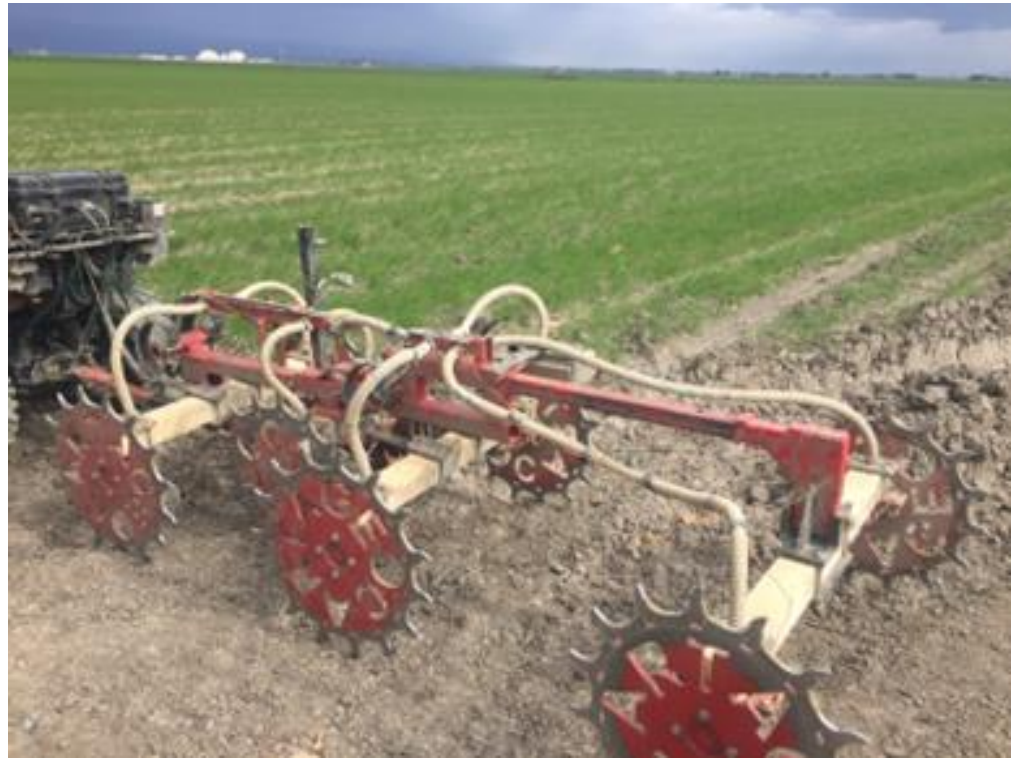
Figure 2. Mobile system to measure the electrical potential difference.
