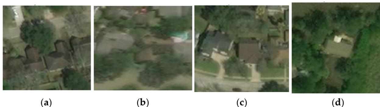
**Figure 10.** Classification and misclassification results. (a) True: undamaged predicted: undamaged; (b) True: damaged predicted: damaged; (c) True: undamaged predicted: damaged; (d) True: damaged predicted: undamaged.
