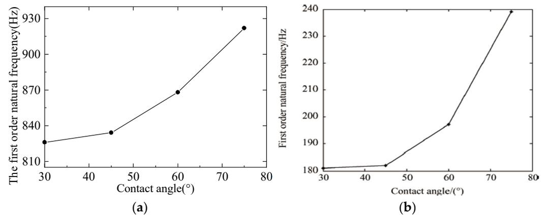
**Figure 12.** Influence of contact angle on the first natural frequency. (a) Model in this paper (b) Model in Ref. [24].
