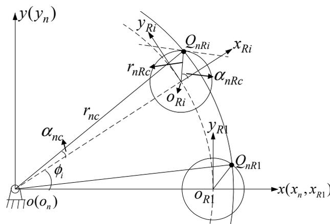
Figure 7. Contact position between the nut and the  $i$ -th roller.
