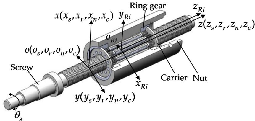
Figure 2. The coordinate system of standard PRSM.
