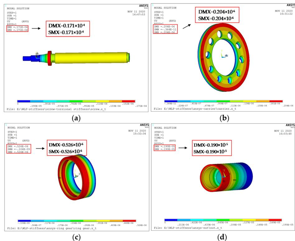
**Figure 9.** Torsional deformation of the component under torque. (a) Torsional deformation of the screw, (b) Torsional deformation of the carrier, (c) Torsional deformation of the ring gear, (d) Torsional deformation of the nut.
