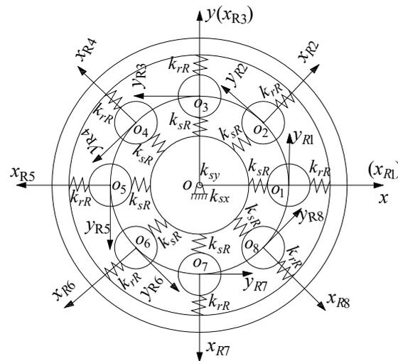
Figure 3. Bending-torsional coupling model of PRSM.
