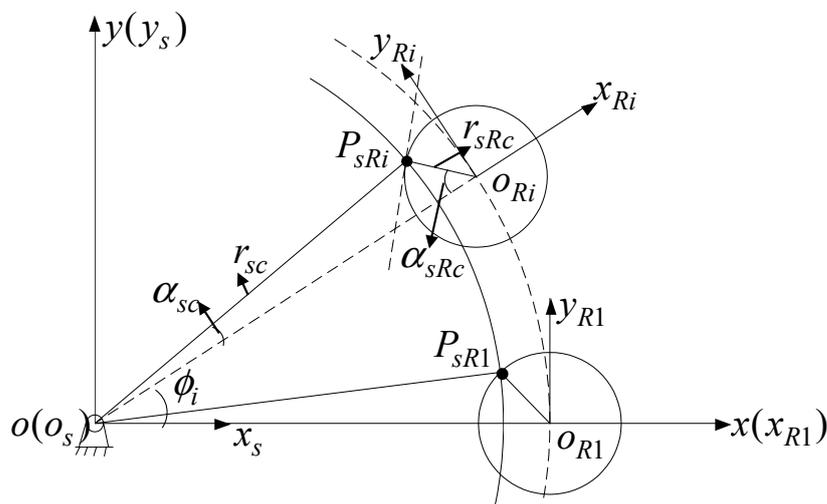
Figure 5. Contact position between the screw and the  $i$ -th roller.
