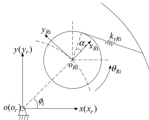
Figure 6. Contact position between the ring gear and the  $i$ -th roller.
