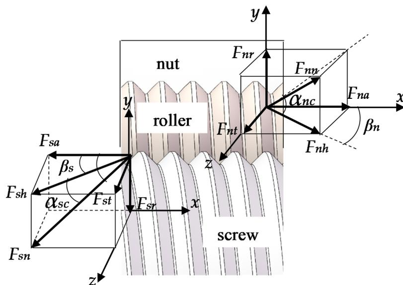
Figure 4. The forces state of thread pairs.
