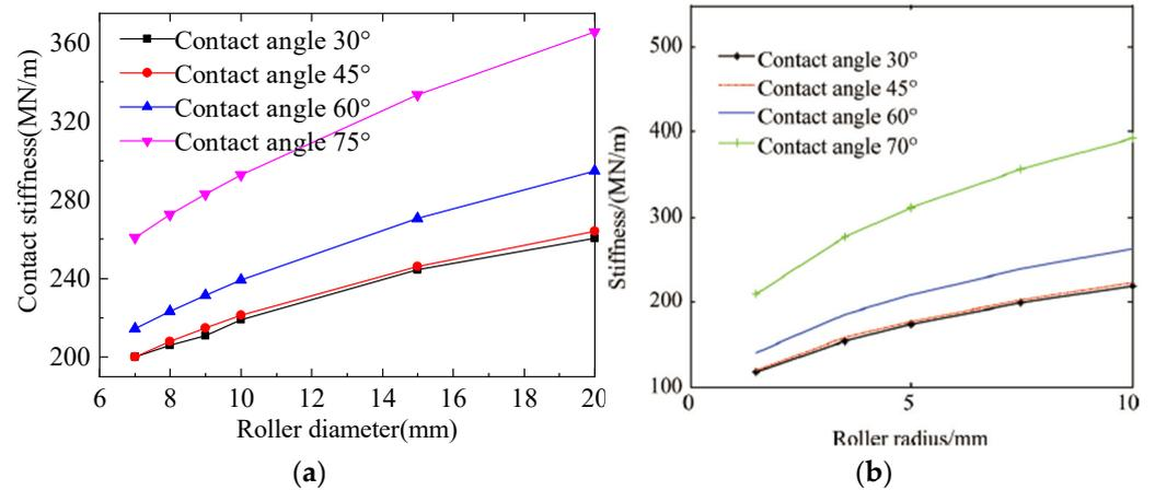
**Figure 10.** The influence of roller radius on contact stiffness. (a) Model in this paper (b) Model in Ref. [24].
