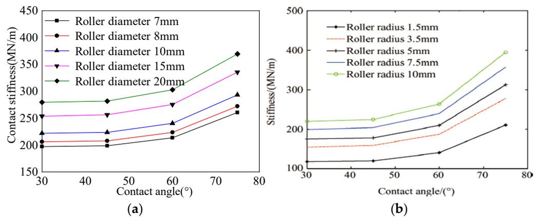
**Figure 11.** The influence of contact angle on contact stiffness. (a) Model in this paper (b) Model in Ref. [24].
