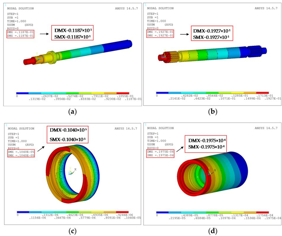
**Figure 8.** Bending deformation of component under radial load. (a) Bending deformation of the screw, (b) Bending deformation of the roller, (c) Bending deformation of the ring gear, (d) Bending deformation of the nut.
