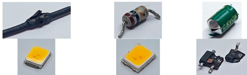
**Figure 7.** Physical failure effects of test components for critical surge levels.
