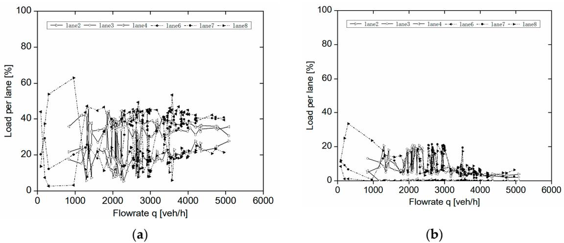
Figure 4. (a) Car load per lane versus flow rate; (b) Truck load per lane versus flow rate.
