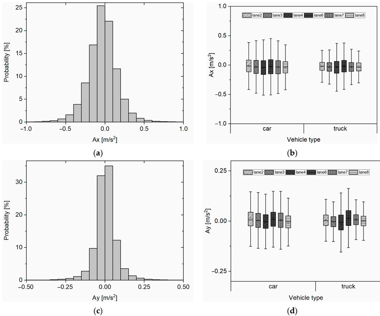
Figure 10. Probability distribution of longitudinal (a) and lateral (b) acceleration; Longitudinal (c) and lateral (d) acceleration for car and truck in different lanes.
