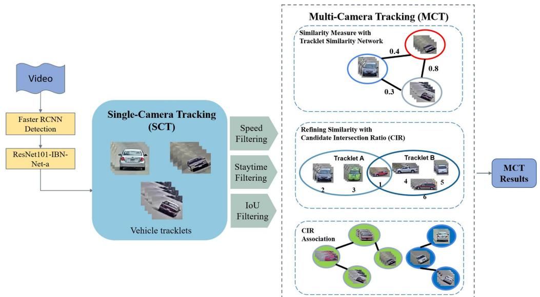
Figure 2. Multi-target multi-camera tracking pipeline.
