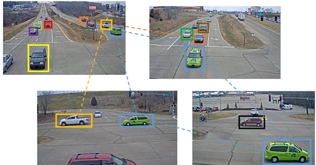
**Figure 1.** A multi-target multi-camera tracking example. The four subfigures show different views captured by cameras. The bounding box with the same color refers to the same car across cameras.
