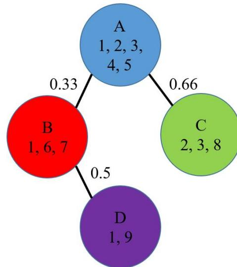
**Figure 5.** A tracklet association example during the execution of the CIR association. Suppose tracklet *B* has the max CIR with tracklet *A*. Since the size of tracklet *B* is smaller than the size of tracklet *A*, tracklet *A* is assigned as tracklet *B*'s parent. We repeat this process and group the tracklets as a tree.
