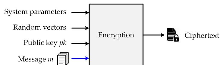
**Figure 2.** Encryption process of a public-key algorithm.
