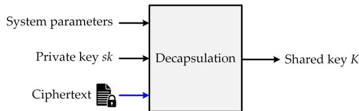
Figure 5. Decapsulation process of a key-establishment algorithm.
