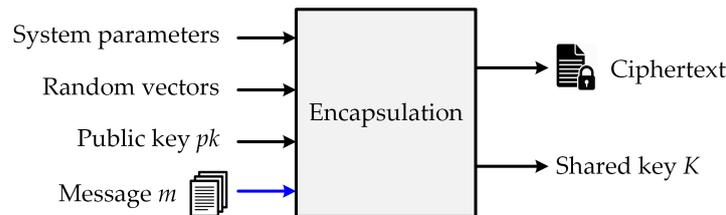
Figure 4. Encapsulation process of a key-establishment algorithm.
