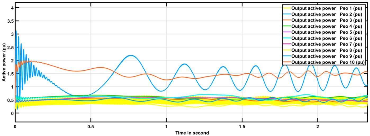
Figure 5. Active power responses without BR and communication delay.
