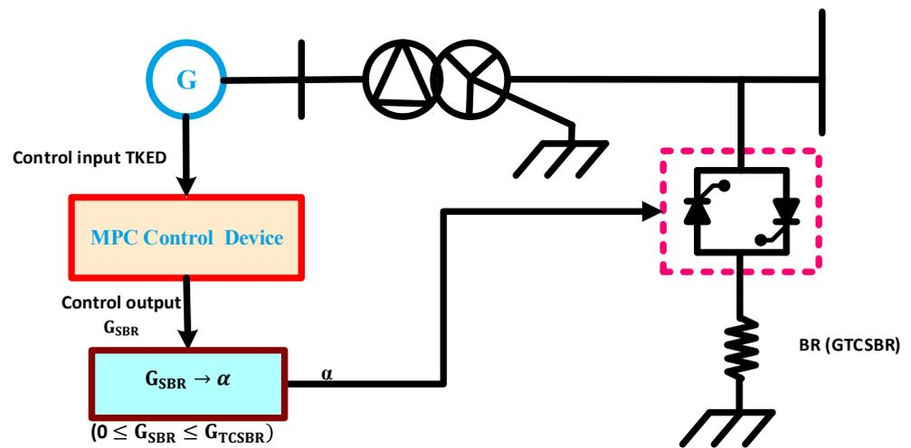
Figure 3. BR with thyristor switching circuit.
