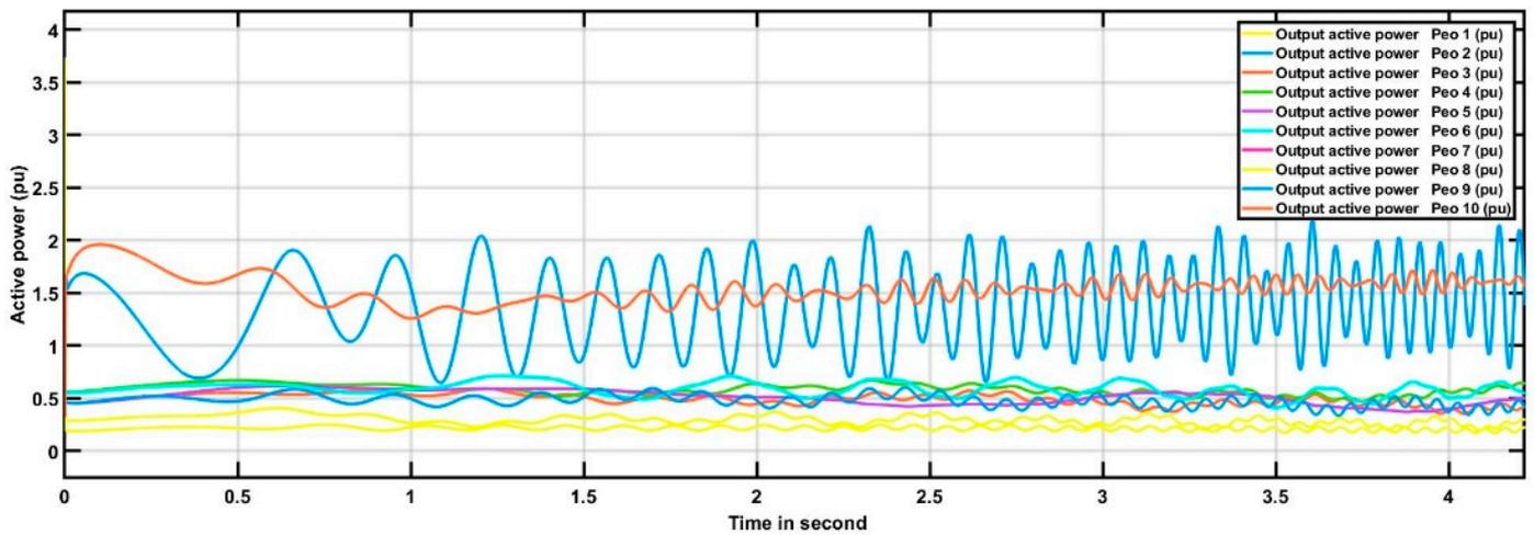
Figure 7. Active power responses with fuzzy controlled BR and communication delay of 20 ms.
