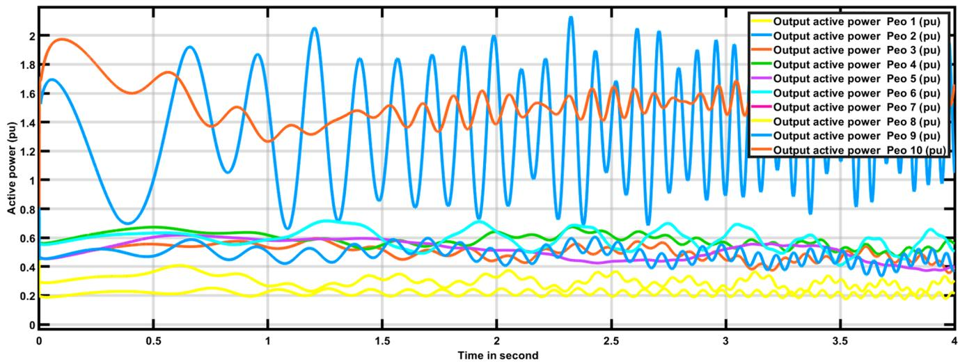
Figure 6. Active power responses with BR and communication delay.
