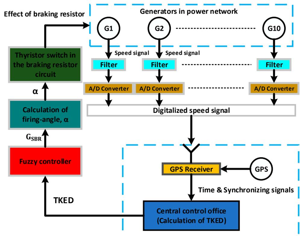
Figure 4. Closed loop control system counting GPS occupation [111].
