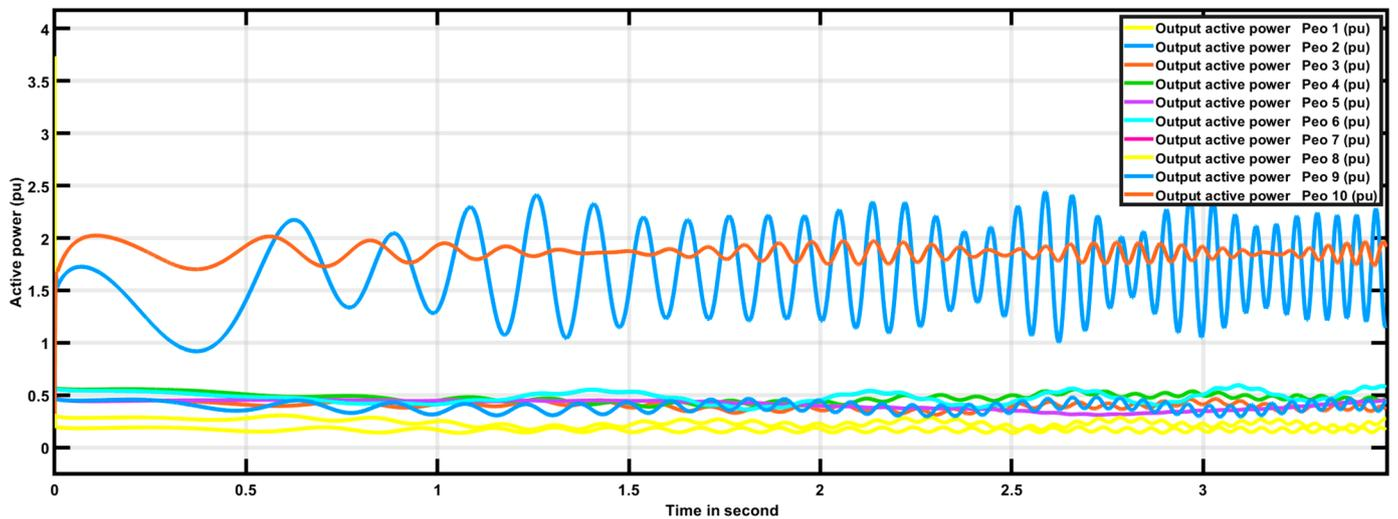
Figure 8. Active power responses with fuzzy controlled BR and communication delay of 300 ms.
