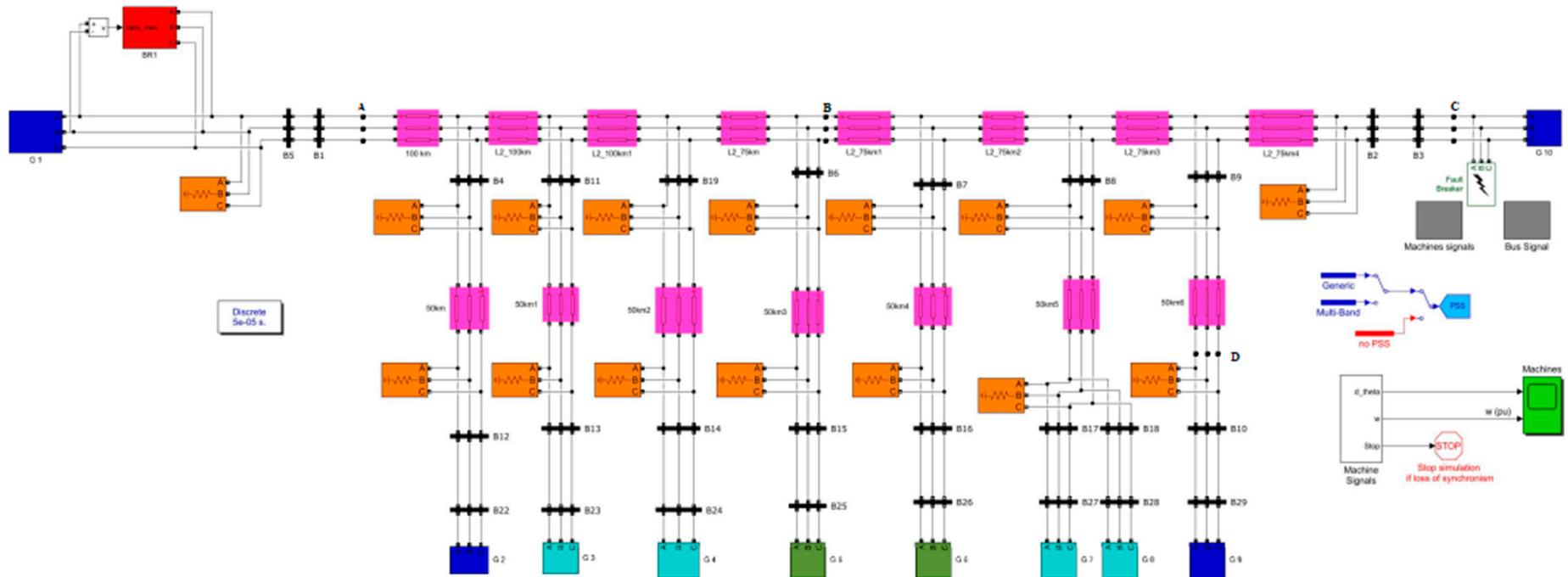
Figure 2. IEEJ WEST 10-machine model.
