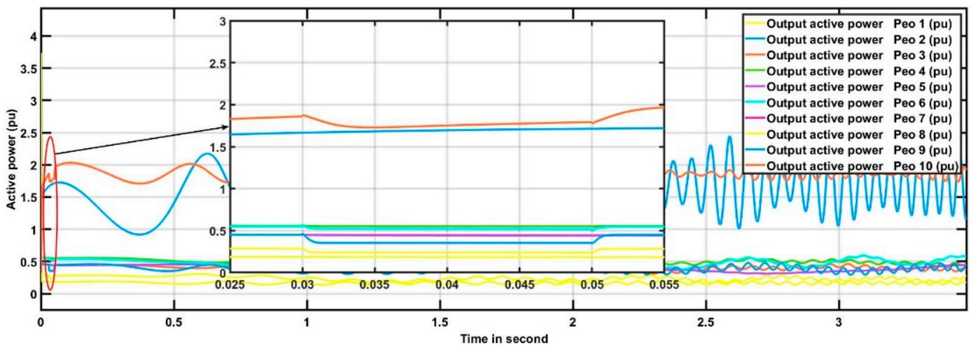
Figure 10. Active power responses for 3 LG fault at point C.
