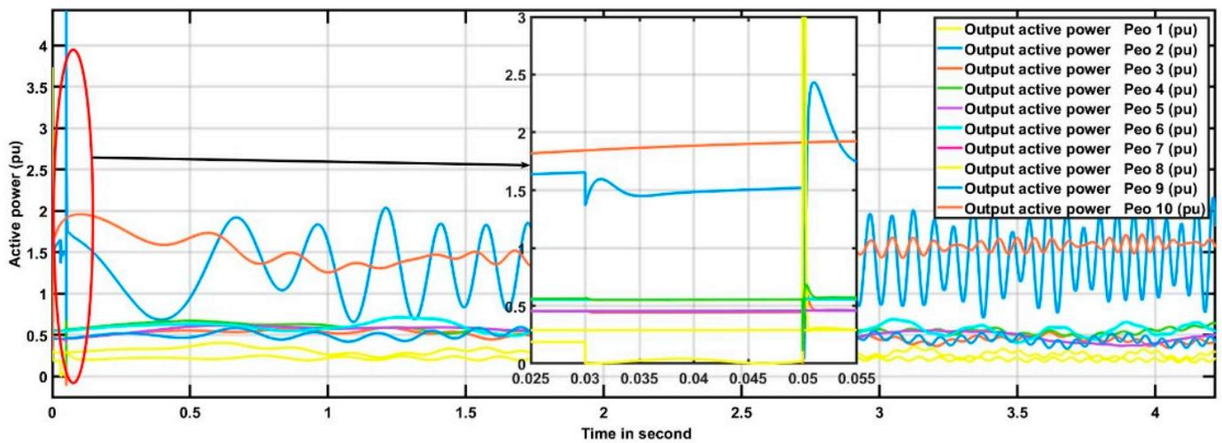
Figure 9. Active power responses for 3 LG fault at point A.
