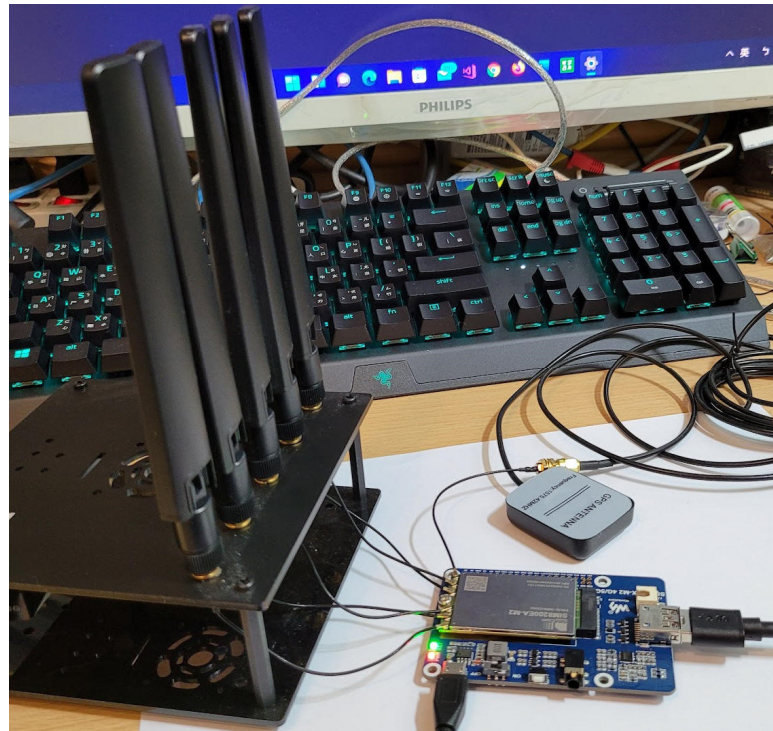
Figure 22. The 5G-dedicated antenna connection used in our experiments.
