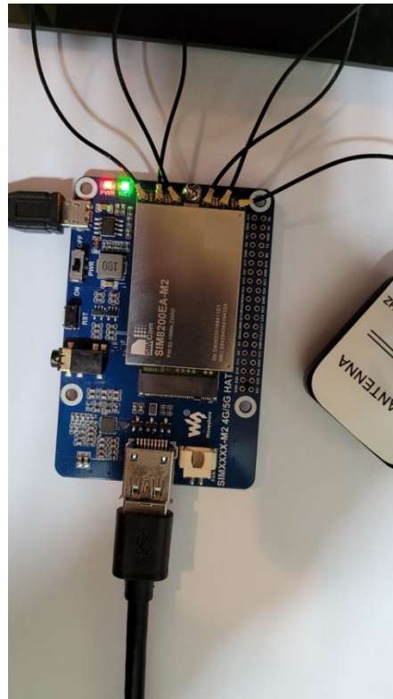
Figure 20. Wiring of SIM8200EA-M2.
