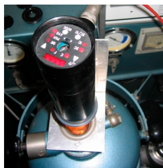
Figure 2. Raytek MR1SC pyrometer installed above the inspection window.
