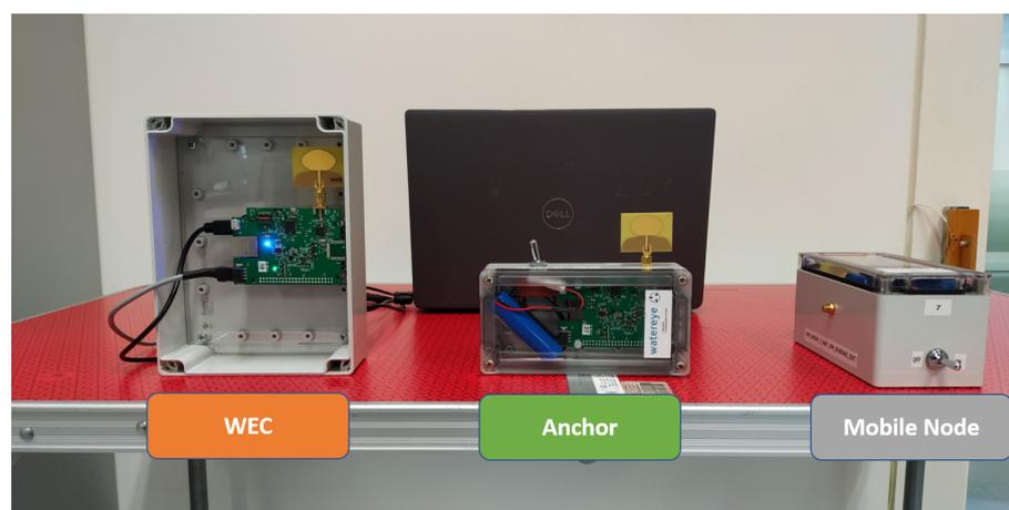
**Figure 15.** Implemented setup for the coverage measurements.
