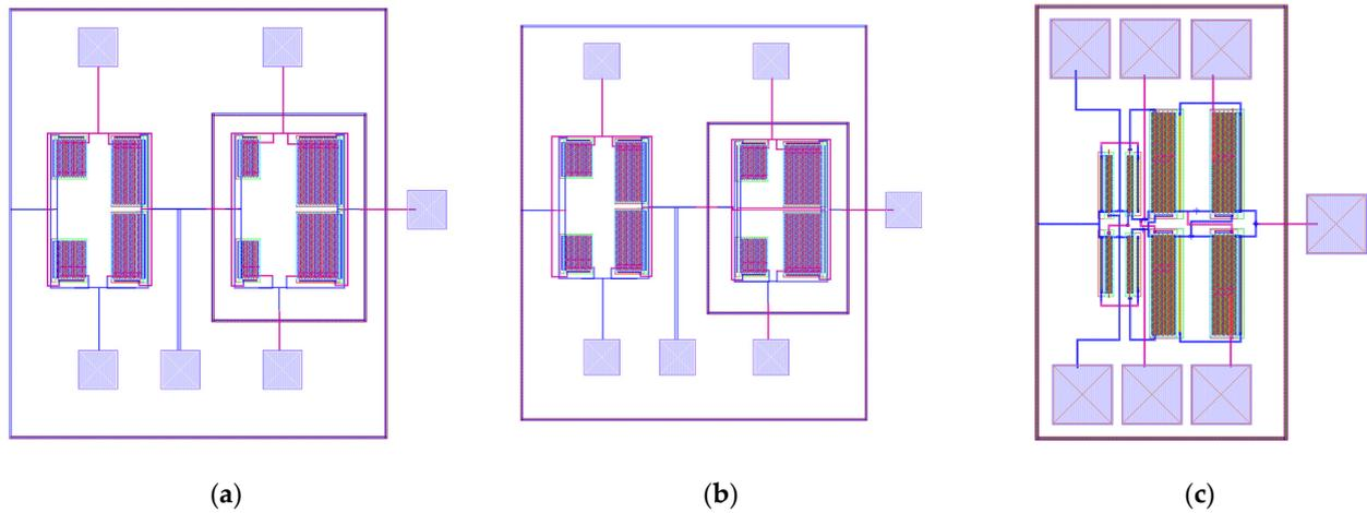
**Figure 5.** Layout of the topology CDC (a), CDB, (b) and CDN (c) in 32 nm with, the iPDK using Cdesigner. The capacitors are not represented because they are occupying much more space in the layout. In practice, the large capacitors can be used in the metal layers.
