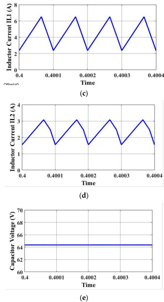
**Figure 6.** Output wave forms of step-up mode. (a) Output voltage, (b) output current, (c) inductor current ( $I_{L1}$ ), (d) inductor current ( $I_{L2}$ ), and (e) capacitor voltage ( $V_{C1}$ ).
