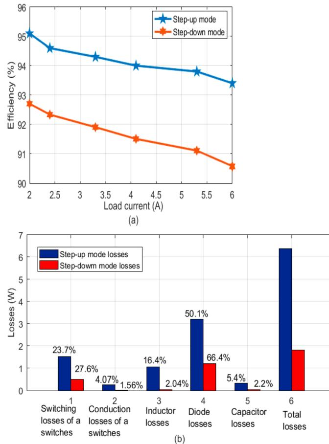
**Figure 11.** Efficiency and loss distributions. (a) Efficiency curve and (b) losses distributions under  $V_0 = 72$  v,  $P_0 = 173$  W.
