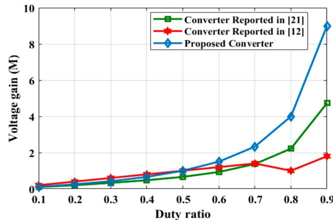
Figure 5. Voltage gain comparison of the proposed converter and similar converters.
