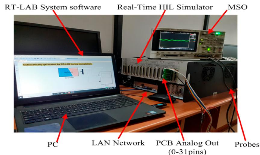
**Figure 8.** HIL experimental set-up of the proposed Zeta converter.
