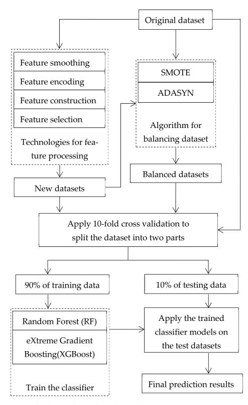
**Figure 1.** The schematic diagram for prediction of CAD.
