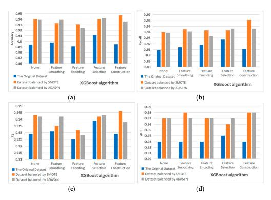
**Figure 5.** Comparison of the effects of four feature processing technologies and two dataset balancing methods on the performance of XGBoost algorithm. (a) In terms of accuracy, (b) In terms of recall, (c) In terms of  $F_1$ , (d) In terms of AUC.
