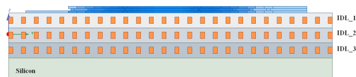
Figure 11. Side view of an inductor containing three layers of DMFs.
