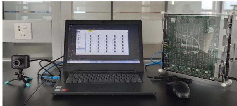
**Figure 5.** Photograph of the designed neuromorphic high-speed object recognition system based on DVS and SpiNNaker. In the system, DVS and SpiNNaker are both configured, controlled and monitored by a laptop.
