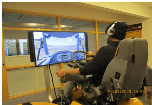
**Figure 4.** Articulated dump truck simulator.
