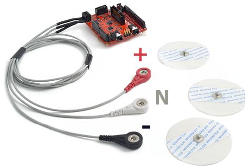
**Figure 2.** ECG electrode connected to e-Health sensor shield.
