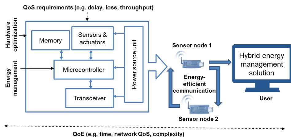
**Figure 2.** Proposed hybrid energy management system for ultra-low power wireless sensor node towards QoS and QoE. (Blue arrow: Connection between sensor node components, Blue filled arrow: Energy-efficient communication between sensor nodes, Black arrow: Energy-efficient techniques applied at the sensor node level, Dotted line: QoE parameter from the QoS requirements to the user satisfaction).
