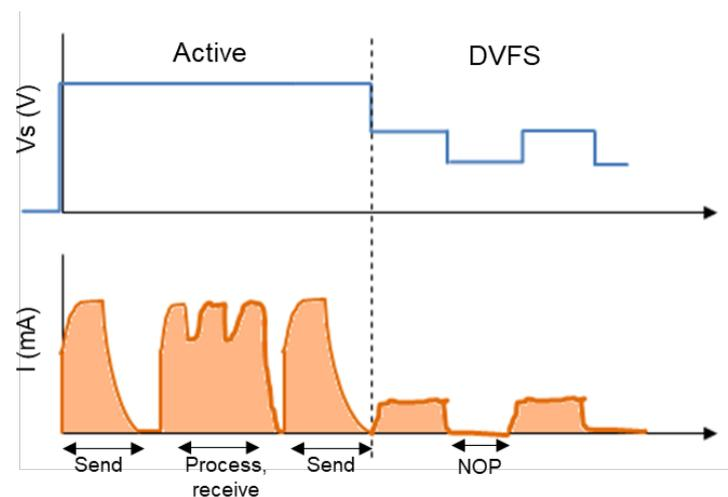
**Figure 9.** Drained current of the microcontroller during active mode (The dotted line defines the end of the active mode. The orange color presents the consumed current for each mode).
