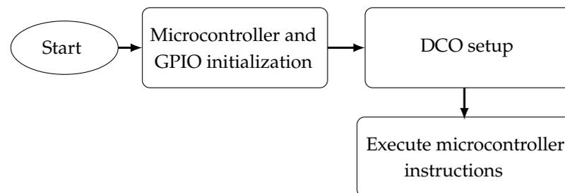
**Figure 3.** Clocking MSP430F5529LP using the internal clock source.
