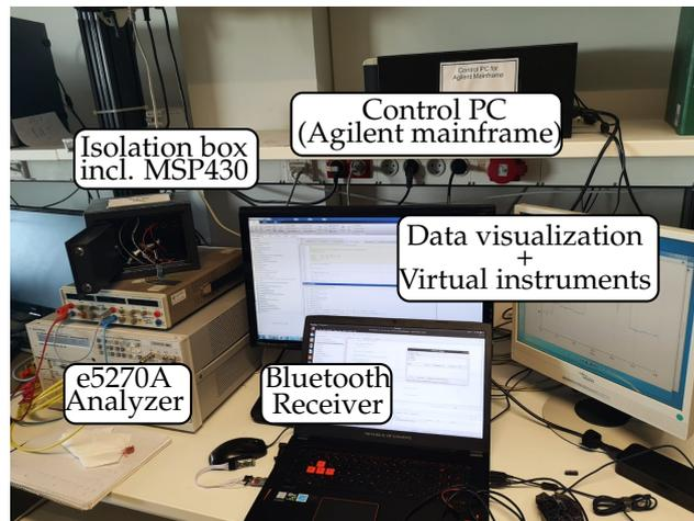
Figure 11. Experimental setup for Bluetooth communication.
