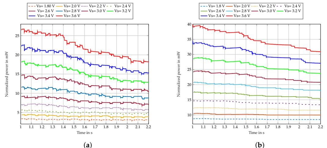
Figure 8. Normalized power during the time for different supply voltages at (a) 6 MHz; (b) 20 MHz.
