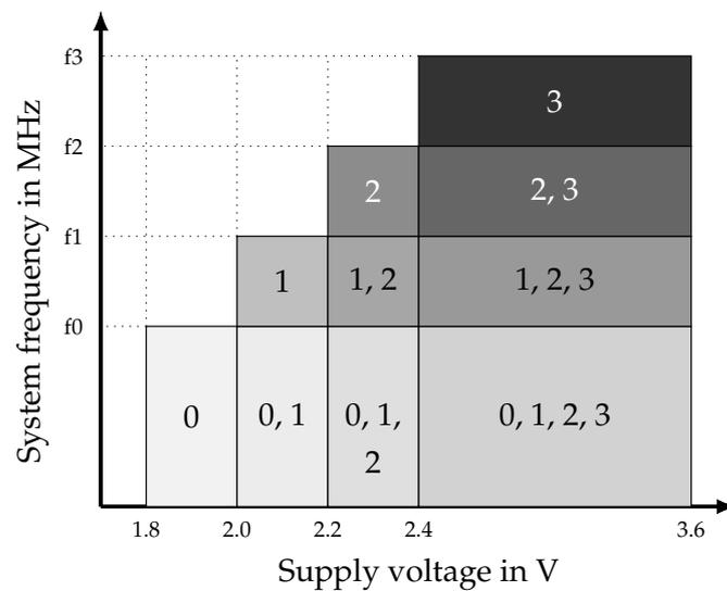
Figure 7. PMM core levels and related frequencies and threshold voltages.
