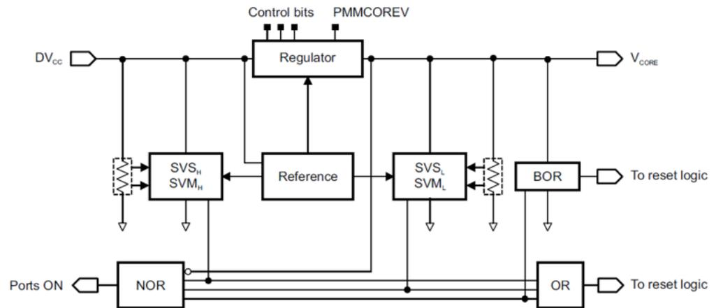
Figure 4. Power management module block diagram following [56].
