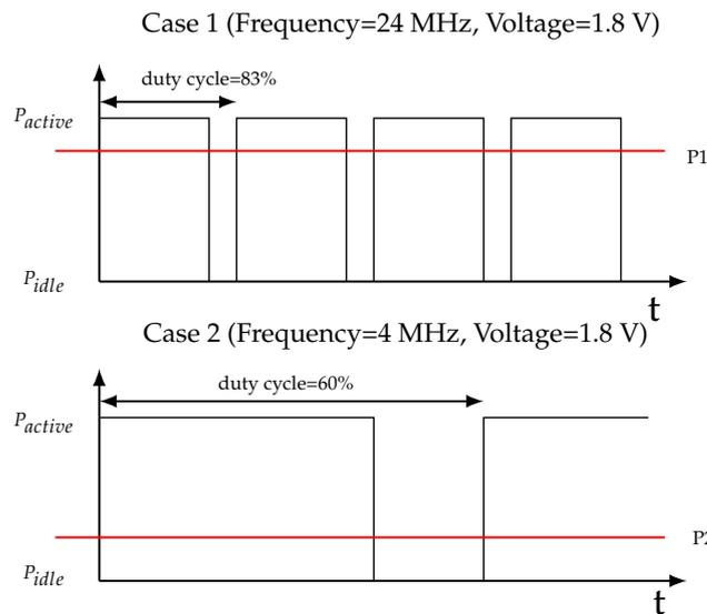
Figure 13. Operating frequency versus power efficiency (P1 and P2 are the average consumed power for high frequency and low frequency, respectively).
