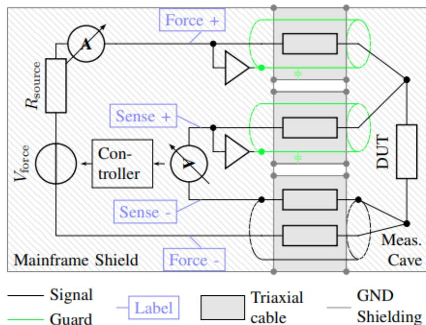
**Figure 6.** Four-wire measurement configuration involving a Keysight Technologies E5270 8-channel precision mainframe.
