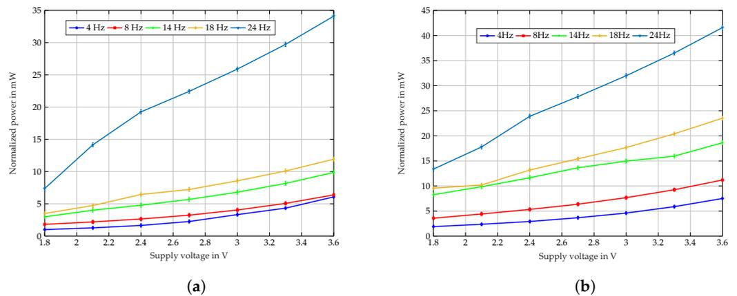
Figure 10. Normalized power vs. supply voltage at various frequencies for (a) “nop” operation; (b) “add” operation.
