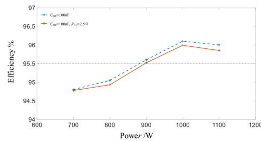
**Figure 14.** Efficiency of the buck converter with DC-side snubbers.
