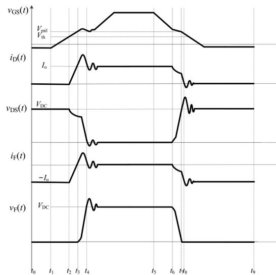
Figure 2. Switching waveforms during the turn-on and turn-off transitions of the SiC MOSFET.
