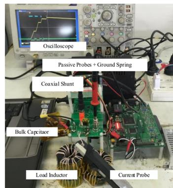
**Figure 9.** DC-side snubber testing platform.
