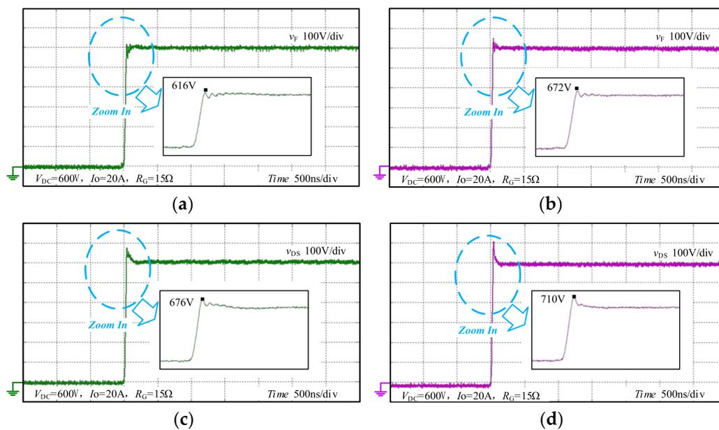
**Figure 11.** Tested waveforms with capacitor C<sub>DE</sub> and resistor R<sub>DE</sub>. (a) Turn-off voltage of the SiC diode at C<sub>DE</sub> = 100 nF and R<sub>DE</sub> = 2.5 Ω, (b) turn-off voltage of the SiC diode at C<sub>DE</sub> = 100 nF and R<sub>DE</sub> = 5 Ω, (c) turn-off voltage of the SiC MOSFET at C<sub>DE</sub> = 100 nF and R<sub>DE</sub> = 2.5 Ω, and (d) turn-off voltage of the SiC MOSFET at C<sub>DE</sub> = 100 nF and R<sub>DE</sub> = 5 Ω.
