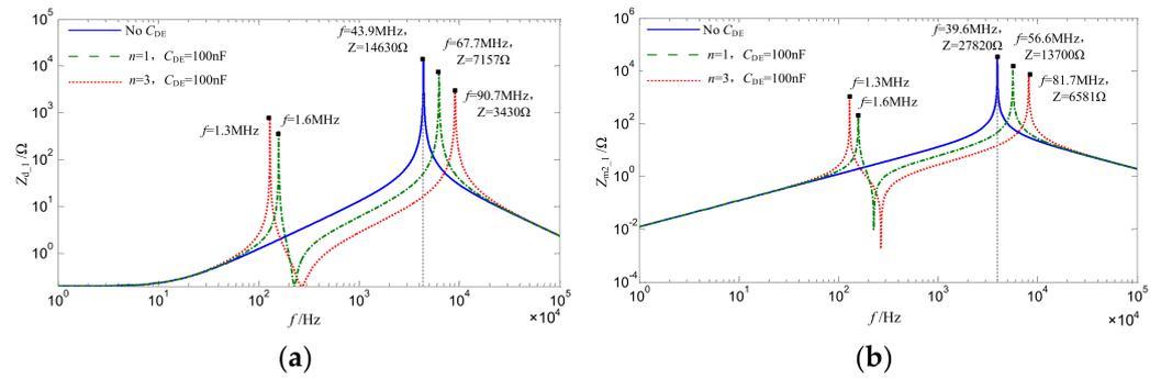
**Figure 5.** Amplitude–frequency curves of terminal impedances,  $Z_{d_1}$  and  $Z_{m2_1}$ , with different  $n$  values (a) at Stage 4 and (b) at Stage 7 and Stage 8.
