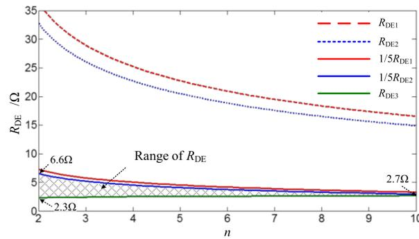
Figure 7. Range of resistor  $R_{DE}$  with different  $n$ .
