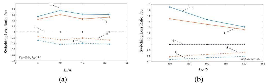
Figure 13. Switching losses of the SiC MOSFET with DC-side snubbers (a) at different  $I_o$  and (b) at different  $V_{DC}$ . (Note: 0: turn-on loss or turn-off loss with no  $C_{DE}$ , 1: turn-on loss with  $C_{DE} = 100$  nF, 2: turn-on loss with  $C_{DE} = 100$  nF and  $R_{DE} = 2.5 \Omega$ , 4: turn-off loss with  $C_{DE} = 100$  nF, 5: turn-off loss with  $C_{DE} = 100$  nF and  $R_{DE} = 2.5 \Omega$ ).
