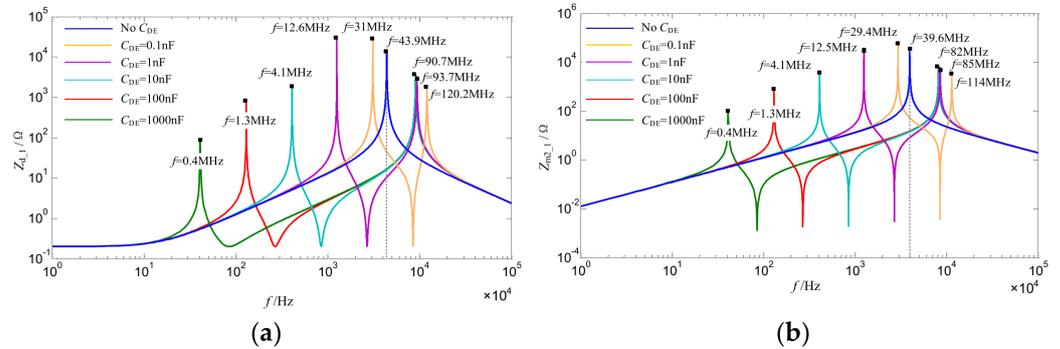
Figure 4. Amplitude–frequency curves of the terminal impedances,  $Z_{d\_1}$  and  $Z_{m2\_1}$ , with different  $C_{DE}$  (a) at Stage 4 and (b) at Stage 7 and Stage 8.
