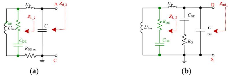
**Figure 6.** Equivalent circuits with capacitor  $C_{DE}$  and resistor  $R_{DE}$  (a) at Stage 4, (b) at Stage 7 and Stage 8.
