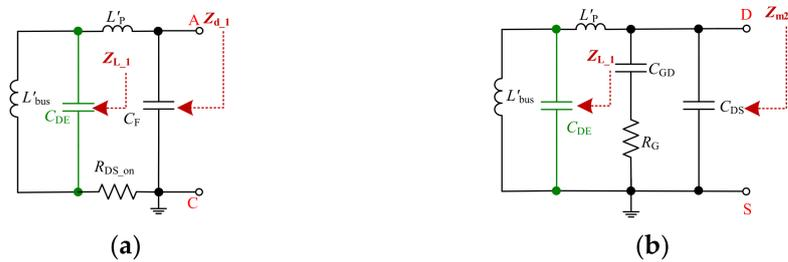
Figure 3. Equivalent circuit with capacitor  $C_{DE}$  (a) at Stage 4 and (b) at Stage 7 and Stage 8.
