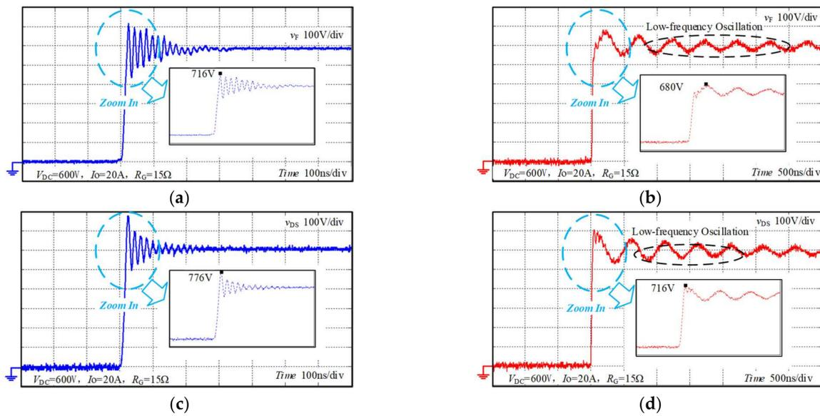
**Figure 10.** Tested waveforms without and with capacitor C<sub>DE</sub>. (a) Turn-off voltage of the SiC diode without C<sub>DE</sub>, (b) turn-off voltage of the SiC diode with C<sub>DE</sub> = 100 nF, (c) turn-off voltage of the SiC MOSFET without C<sub>DE</sub>, and (d) turn-off voltage of the SiC MOSFET with C<sub>DE</sub> = 100 nF.
