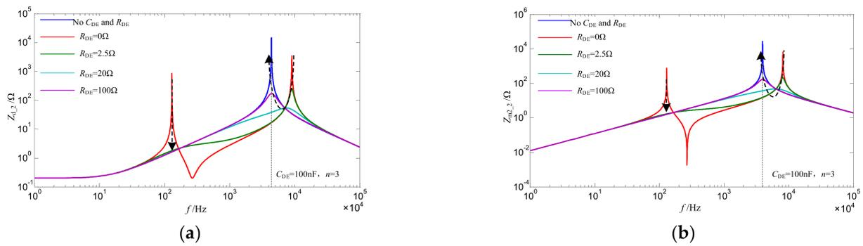
**Figure 8.** Amplitude–frequency curves of the terminal impedances,  $Z_{d\_2}$  and  $Z_{m\_2}$ , with capacitor  $C_{DE}$  and resistor  $R_{DE}$  (a) at Stage 4 and (b) at Stage 7 and Stage 8.
