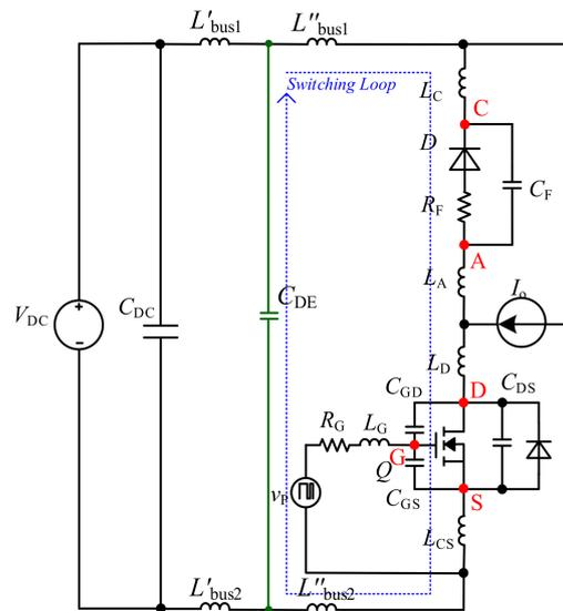
Figure 1. Phase-leg configuration with DC-side Snubber  $C_{DE}$ .
