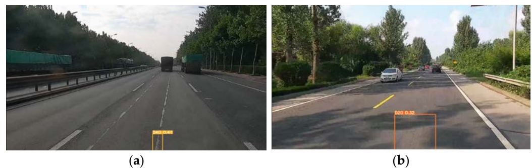
Figure 8. False detection results of pavement cracks: (a) longitudinal crack was mistakenly detected as pothole; (b) longitudinal crack was mistakenly detected as alligator crack.
