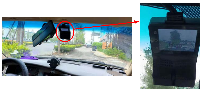
Figure 1. The high-resolution camera installed in a car to collect data of pavement cracks.
