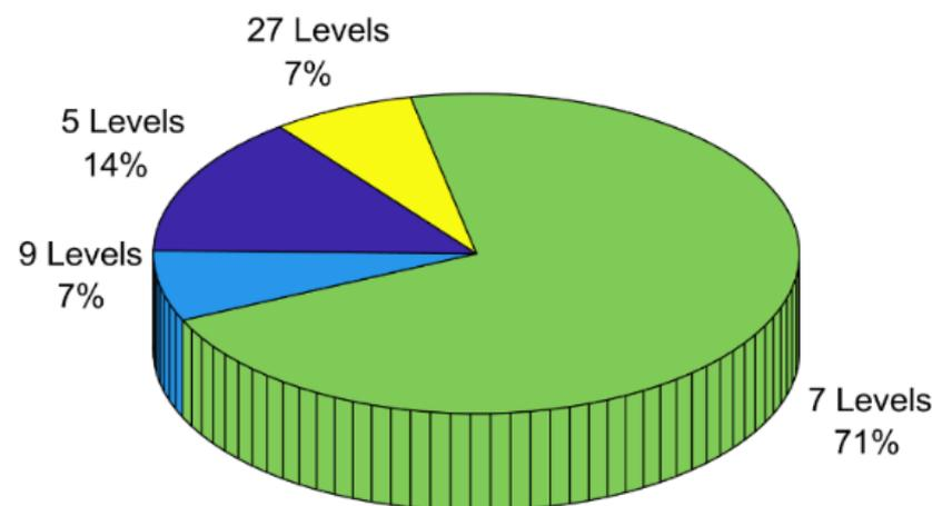
**Figure 8.** The graph represents the number of levels most commonly used by multilevel inverters.
