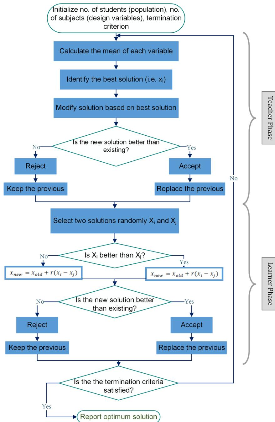
Figure 3. Flowchart of the TLBO algorithm [18].
