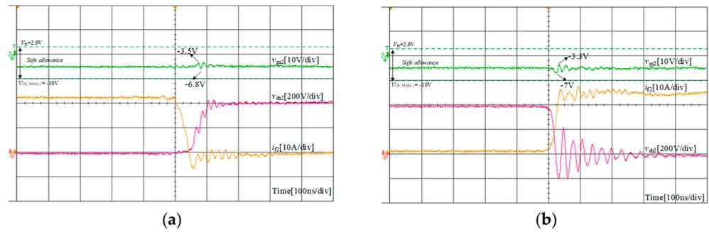
Figure 10. Experimental results with the proposed driver. (a) during  $Q_1$  turn-ON transition, and (b) during  $Q_1$  turn-OFF transition.
