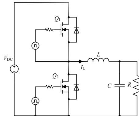
Figure 1. Synchronous buck converter.
