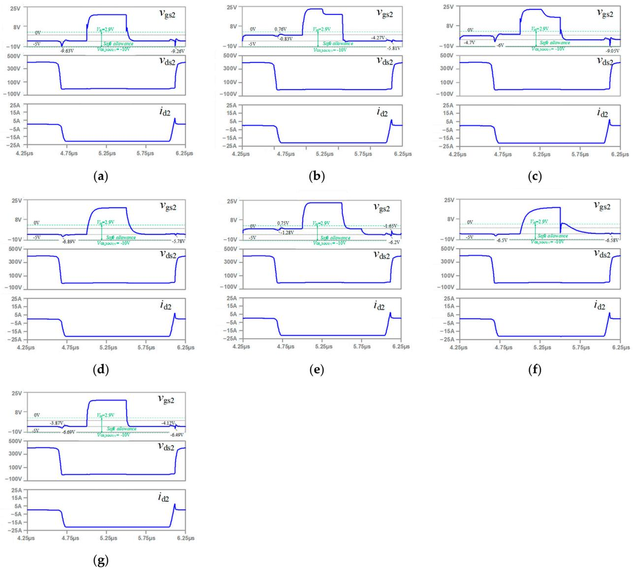
**Figure 8.** Simulation results of the prior drivers in [24–27,30,31] and the proposed driver. (a) the conventional driver in [24], (b) driver in [25], (c) driver in [26], (d) driver in [27], (e) driver in [30], (f) driver in [31] and (g) the proposed driver.
