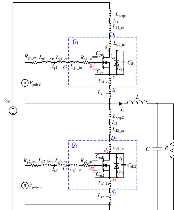
Figure 2. Synchronous buck considering the parasitic parameters.
