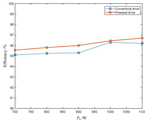
Figure 12. Efficiency of synchronous buck with the conventional driver and the proposed driver.
