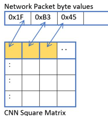
**Figure 3.** Mapping packet byte values into pixels (Recreated with permission from ref. [14]. Copyright 2022 IEEE).
