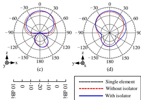
**Figure 11.** Radiation patterns of a field-domain SICS [58]. (a) State 1, xz plane, (b) State 1, yz plane, (c) State 2, xz plane, (d) State 2, yz plane.
