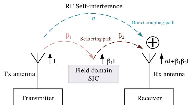
Figure 9. Operation mechanism of the FDSIC.
