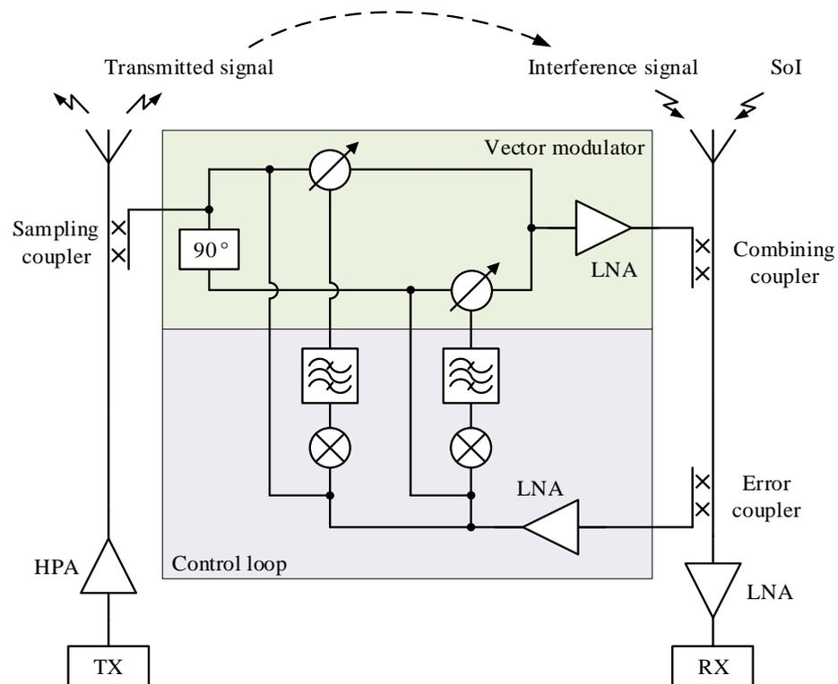
**Figure 5.** A typical analog SIC topology.
