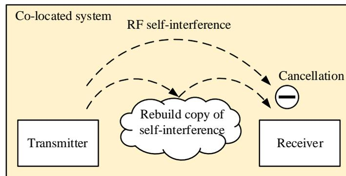
Figure 2. Operation mechanism of the SIC techniques.
