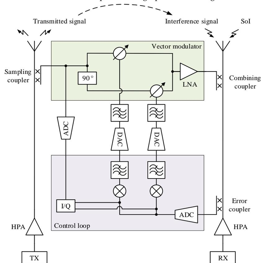
**Figure 8.** A typical analog–digital hybrid SIC topology.
