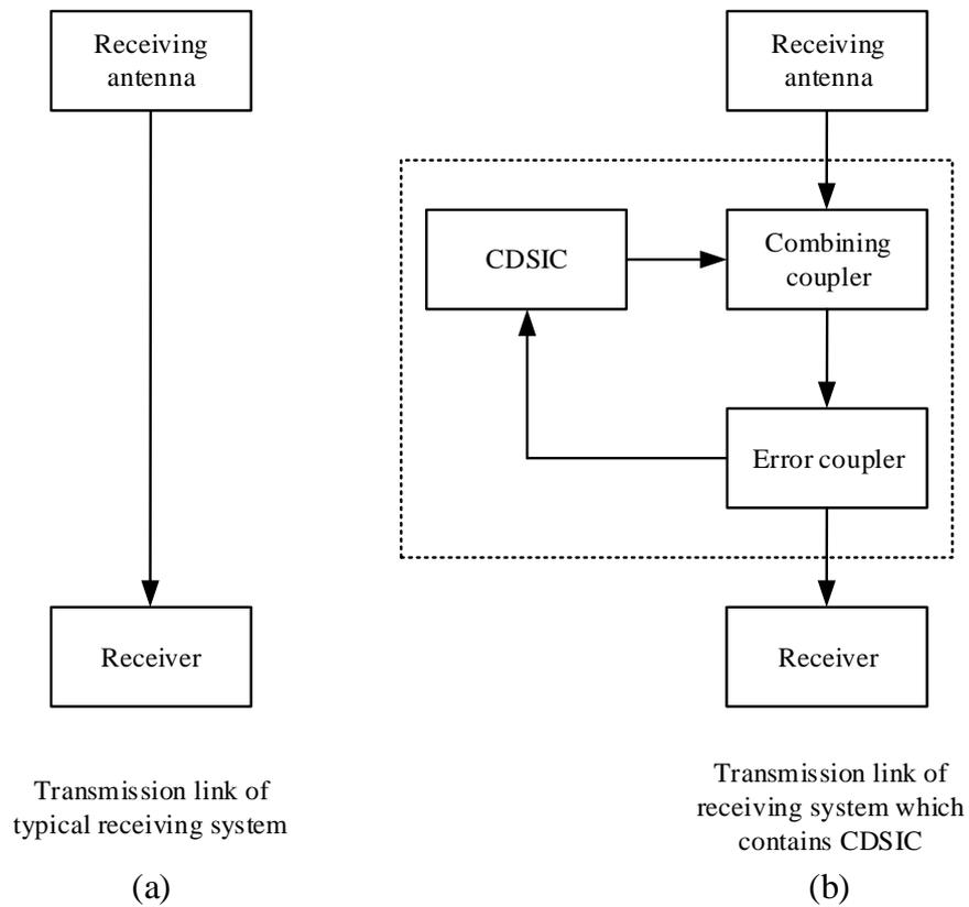
Figure 13. Typical receiving system and receiving system containing a CDSIC.
