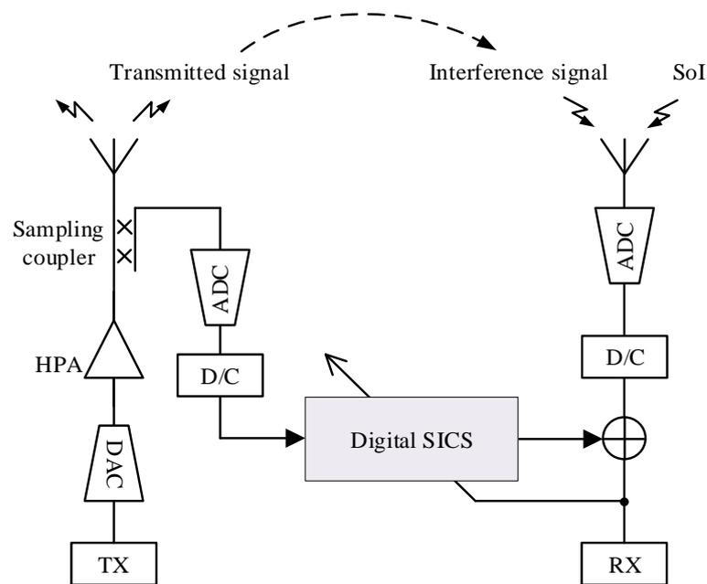
Figure 6. A typical digital SIC topology.
