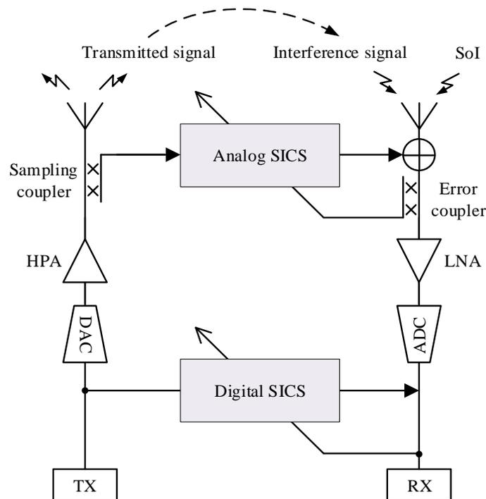
Figure 7. A two-stage SIC topology that contains both the analog SIC and digital SIC.
