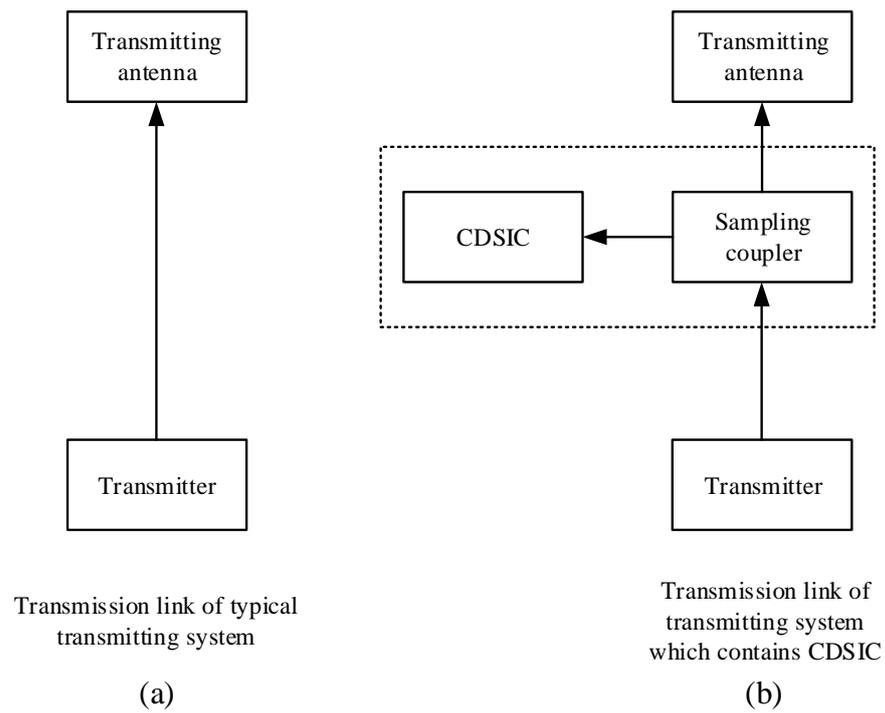
Figure 12. Typical transmitting system and transmitting system containing a CDSIC.
