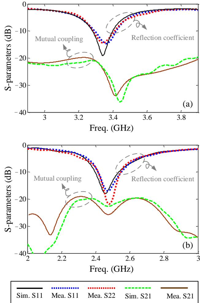
Figure 10. S-parameter performance of a field-domain SICS [58]. (a) State 1, (b) State 2. The dashed lines indicate the measurement results, the solid lines indicate the simulation results.
