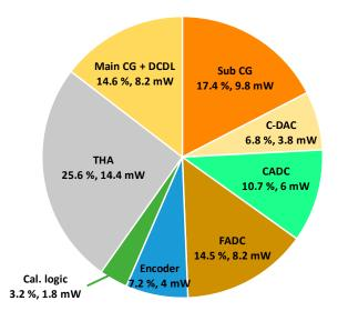
Figure 19. Power breakdown.
