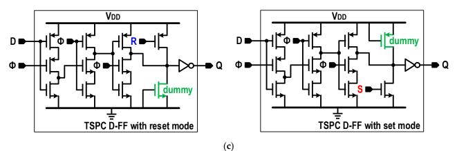
**Figure 9.** Main clock generator. (**a**) Multi-phase generation logic. (**b**) Timing diagram. (**c**) Circuits for the TSPC DFF with set and reset modes.
