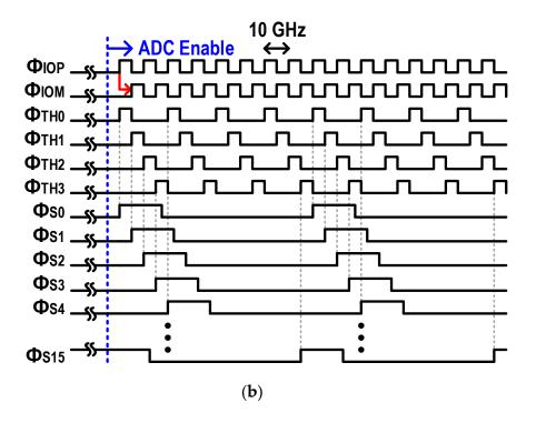
Figure 1. Proposed 6-bit 20 GS/s TI two-step flash ADC. (a) Block and (b) timing diagrams.
