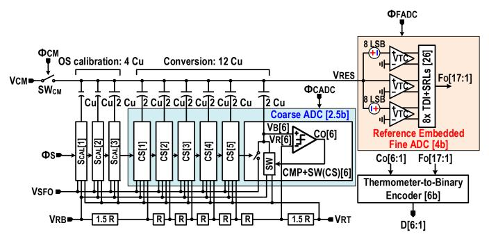
Figure 3. Block diagram of the 6-bit 1.25 GS/s two-step flash ADC.
