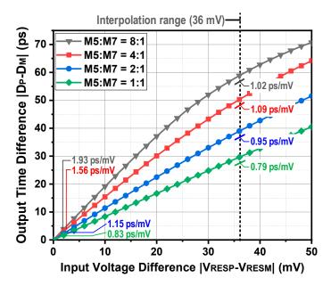
**Figure 7.** Output time difference of the VTC,  $D_P$ - $D_M$ , versus various input voltages,  $V_{RESP}$ - $V_{RESM}$ , according to the size ratios of M5 and M7 of the VTC.
