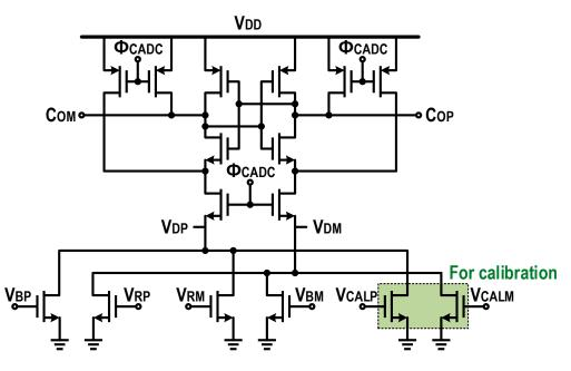
Figure 5. Pseudo differential comparator with the offset calibration capability used in the CADC.
