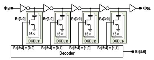
Figure 10. Block diagram of 6-bit DCDL.
