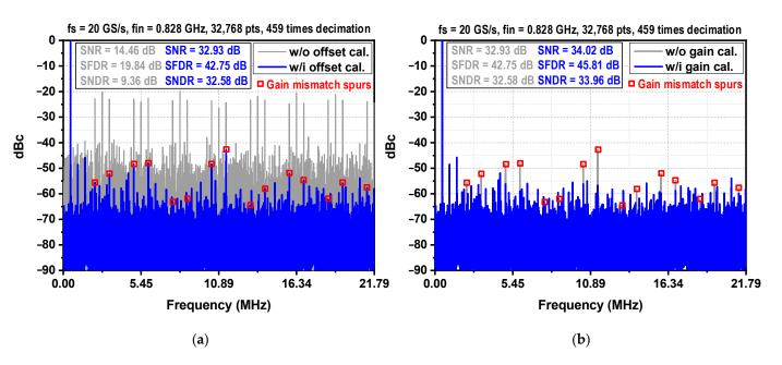
on [28], and as a result, SNR, SFDR, and SNDR were improved to 34.02, 45.81, and 33.96 dB, respectively, as shown in Figure 16b.
