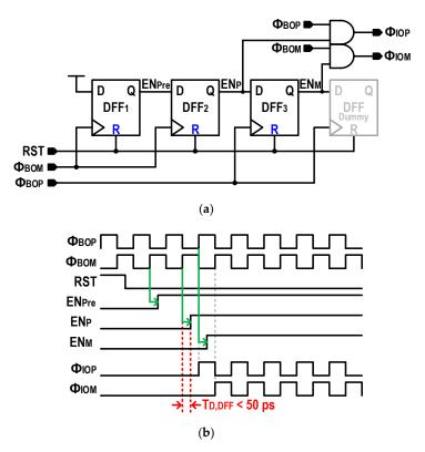
Figure 8. Clock initial logic. (a) Block and (b) timing diagrams.
