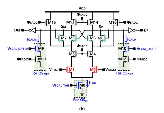
**Figure 6.** (a) Four-bit 8-time time-domain interpolating FADC. (b) Reference-embedded VTC with positive feedback for gain boosting.
