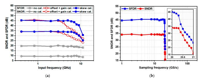
**Figure 18.** Measured SNDR and SFDR versus various (**a**) input frequencies at 20 GS/s and (**b**) conversion rates with a 0.828 GHz input frequency.
