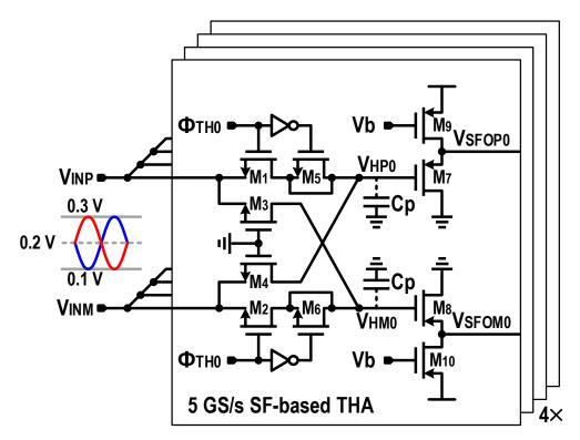
**Figure 2.** Input network of the proposed 20 GS/s TI ADC composed of 4-channel 5 GS/s SF-based THAs.
