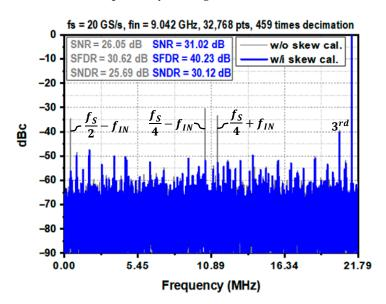
**Figure 17.** Measured FFT spectrum with and without skew calibration at 20 GS/s with a 9.085 GHz input.
