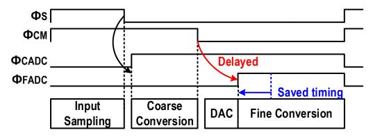
Figure 4. Timing diagram of the 6-bit 1.25 GS/s two-step flash ADC.
