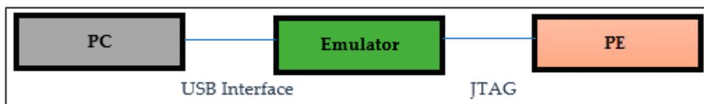
Figure 5. Environmental setup of emulator.
