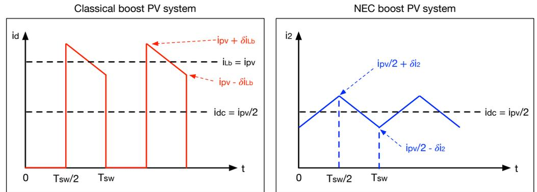
Figure 5. Waveforms of the output currents of classical boost and NEC boost PV systems ( $d = 0.5$ ).
