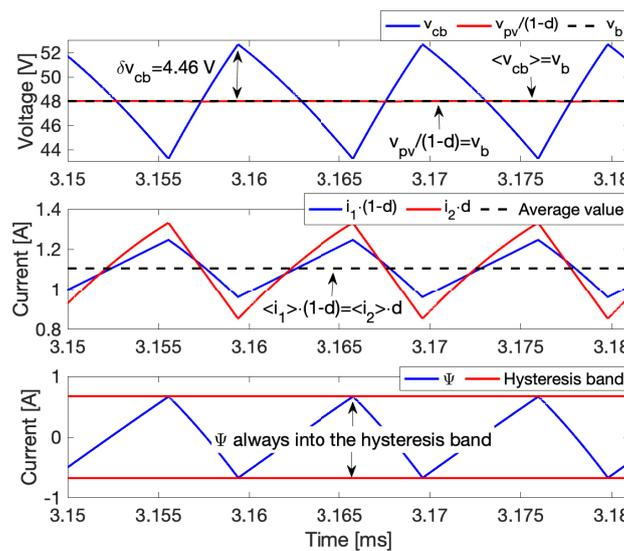
Figure 16. Stable operation of the proposed PV system.
