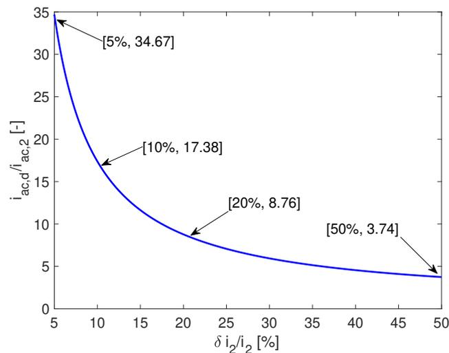
**Figure 6.** Comparison of the AC components introduced into the second stage by both the classical and NEC boost solutions ( $d = 0.5$ ).
