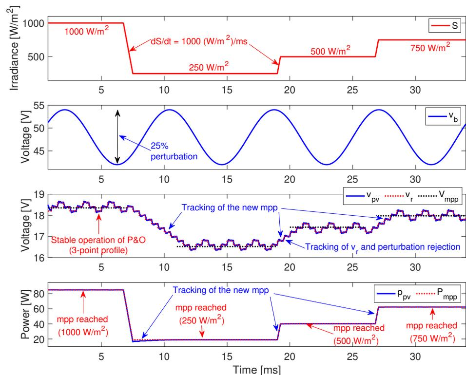
**Figure 18.** Complete PV system operation under changing irradiance conditions.
