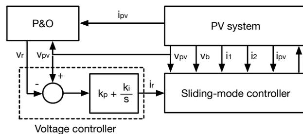
Figure 10. Complete control structure.
