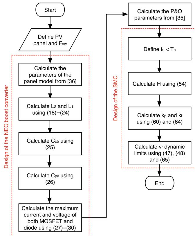
**Figure 13.** Design process for both the NEC boost converter and SMC.
