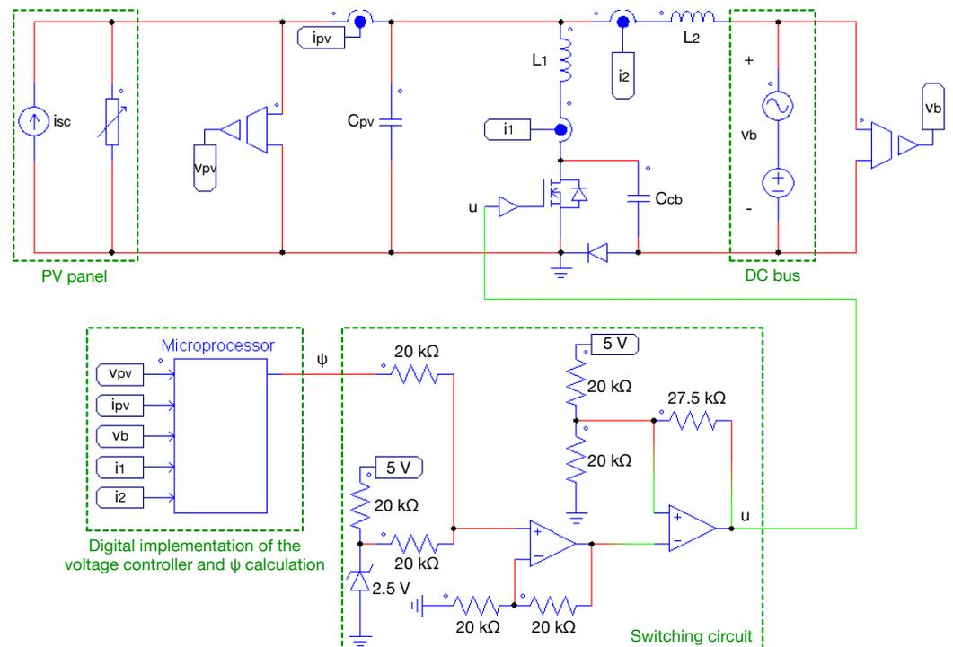
Figure 14. PV system circuit implemented in PSIM.
