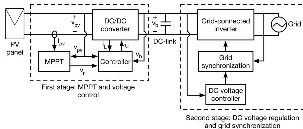
**Figure 1.** Structure of a PV microinverter with DC-link regulation and grid connection.
