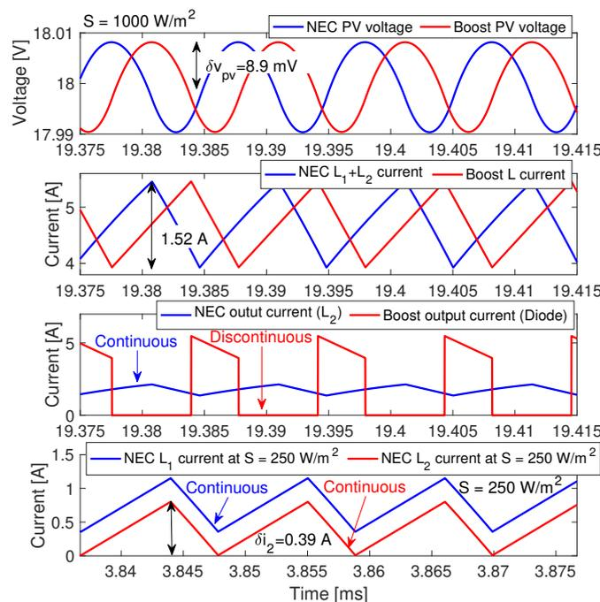
**Figure 15.** Steady-state operation of the PV system and comparison with the classical boost topology.
