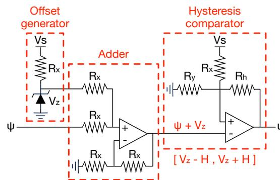
Figure 9. Switching circuit implementing the control law (51).
