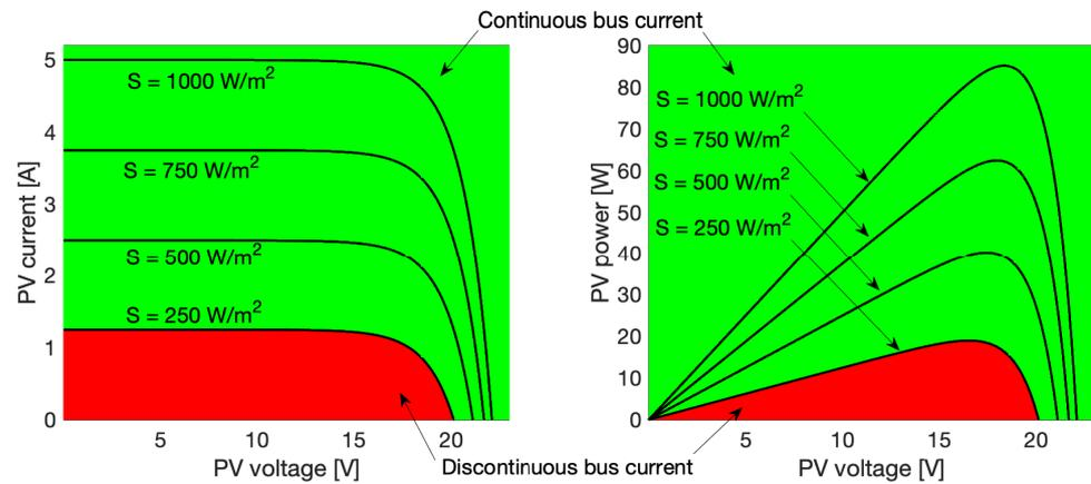
Figure 12. Electrical characteristics of the PV panel.
