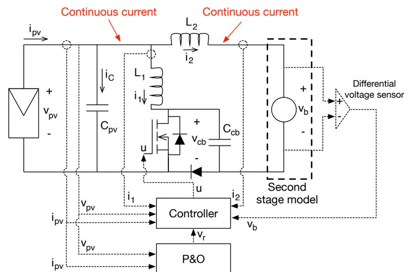
**Figure 2.** Circuitual description of the PV system based on the NEC boost converter.
