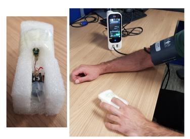
Figure 5. An example of BP and PPG setup for data acquisition on volunteers at STMicroelectronics.
