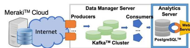
**Figure 1.** The connection architecture of the Wi-Fi network and computing services for data processing.
