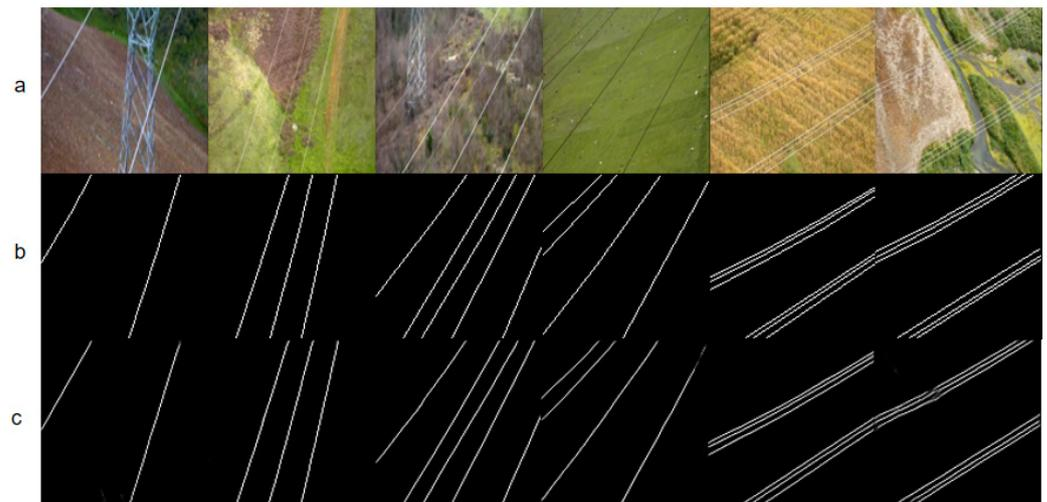
**Figure 10.** The PLE results with typical background. (a) Power line images. (b) Ground truth labels. (c) PLE results based on the proposed model.
