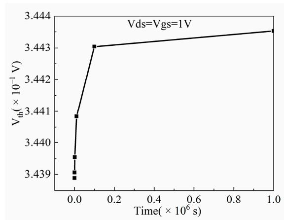
**Figure 9.** The threshold voltage variation of NFinFET under HCl for different times.
