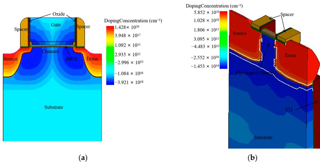
**Figure 1.** The device structures. (a) The structure of planar NMOS; (b) the cross-section view of NFinFET.
