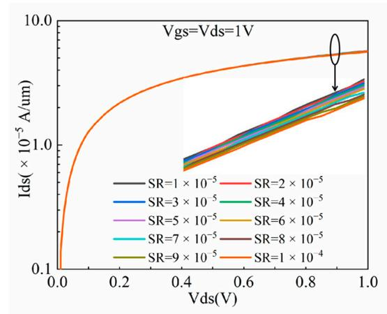
**Figure 7.** The saturation current variation of NFinFET under different surface resistances.
