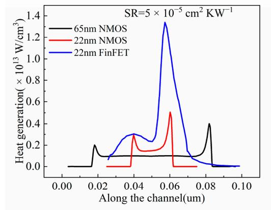
**Figure 3.** The heat profiles for different devices along the channel.
