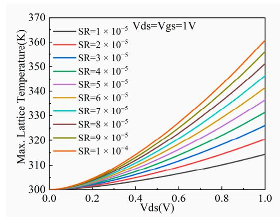
**Figure 8.** The maximum lattice temperature variation of NFinFET under different surface resistances.
