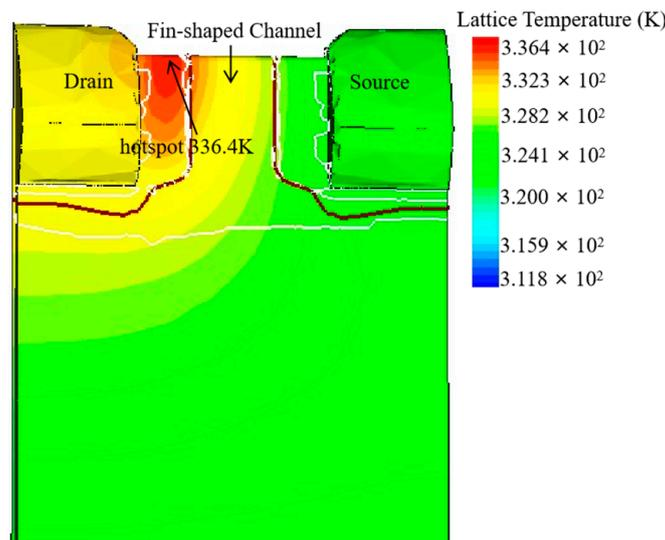
Figure 5. The temperature distribution of NFinFET with  $SR = 5 \times 10^{-5} \text{ cm}^2 \text{ KW}^{-1}$ .
