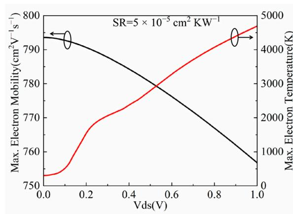
**Figure 4.** The maximum electron temperature and electron mobility of NFinFET against the drain voltage.
