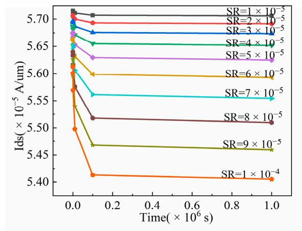
**Figure 12.** The saturation current variations of NFinFET against time at different SRs.
