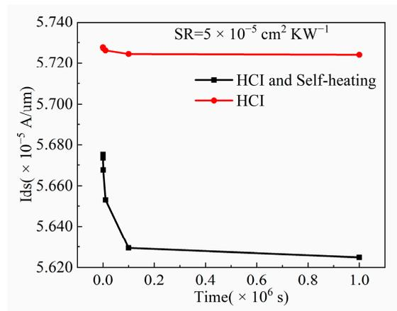
**Figure 11.** Comparison of results of the saturation current of NFinFET between HCl and HCl with self-heating effect at different time.
