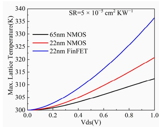
**Figure 2.** The lattice temperature profiles for different devices.
