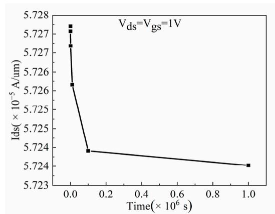
**Figure 10.** The saturation current variation of NFinFET under HCl for different times.
