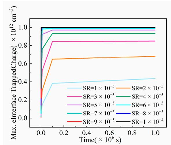
Figure 13. The maximum interface trapped charge variation of NFinFET against time at different SRs.
