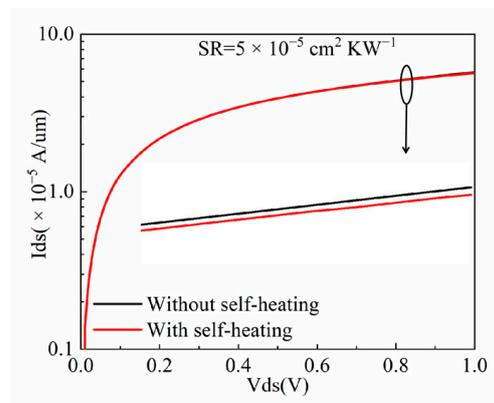
Figure 6. Comparison of the drain current for an NFinFET without the self-heating effect and an NFinFET under the self-heating effect.
