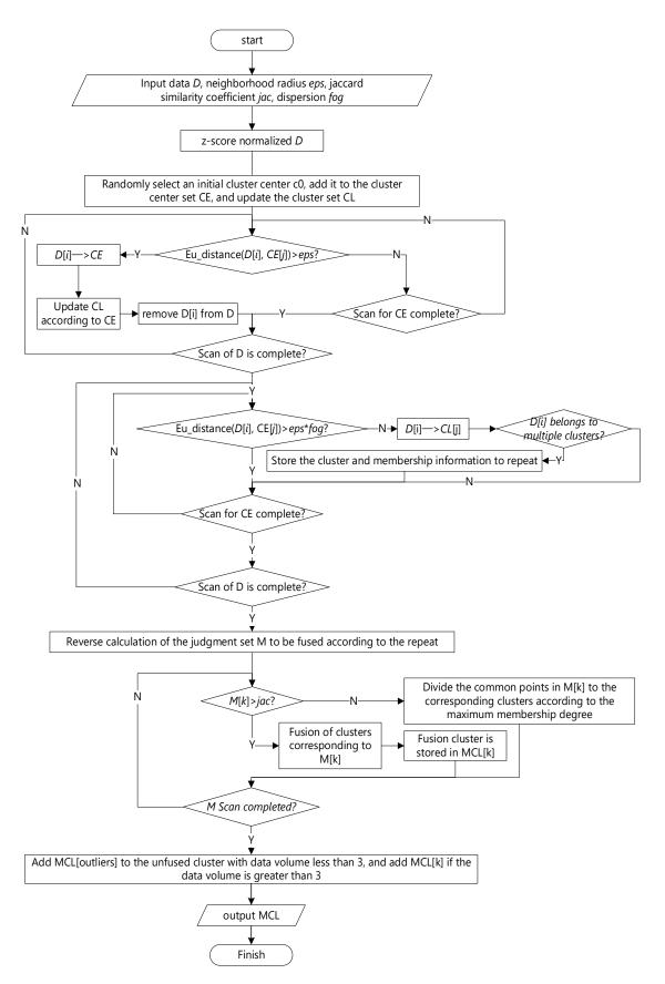
Figure 2. PRI-MFC algorithm flow chart.
