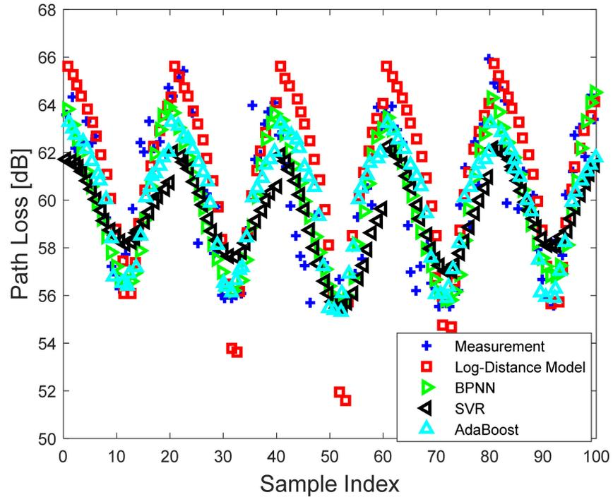
**Figure 5.** Path loss prediction performance of machine learning algorithms using 100 sample data for OSRC base station operating at 96.5 MHz. Note: For sample data of OSRC, only 30 computed samples were used in the training.
