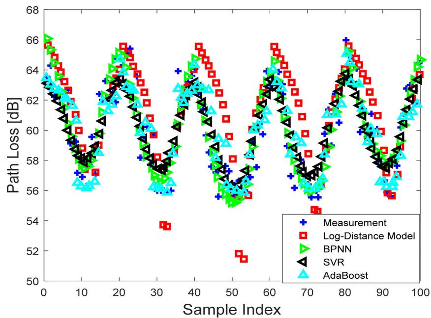
**Figure 6.** Path loss prediction performance of machine learning algorithms using 100 sample data for OSRC base station operating at 96.5 MHz. Note: 30 computed and 30 measured samples were used during the training.
