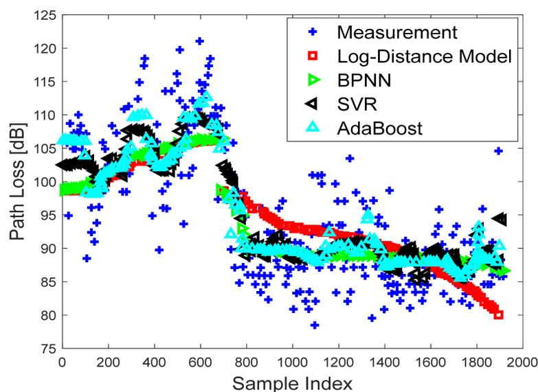
**Figure 3.** Path loss prediction of various machine-learning algorithms on the test dataset using samples from OSRC base station; 80% of data were used for training while the other 20% for tests.
