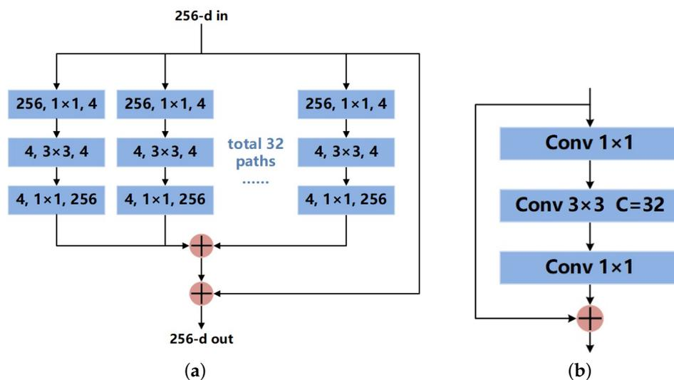
Figure 3. Residual block structure of ResNeXt50: (a) theoretical structure; (b) practical structure.
