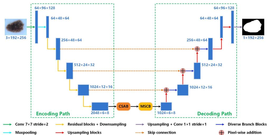
Figure 2. Diagram of the proposed network structure.
