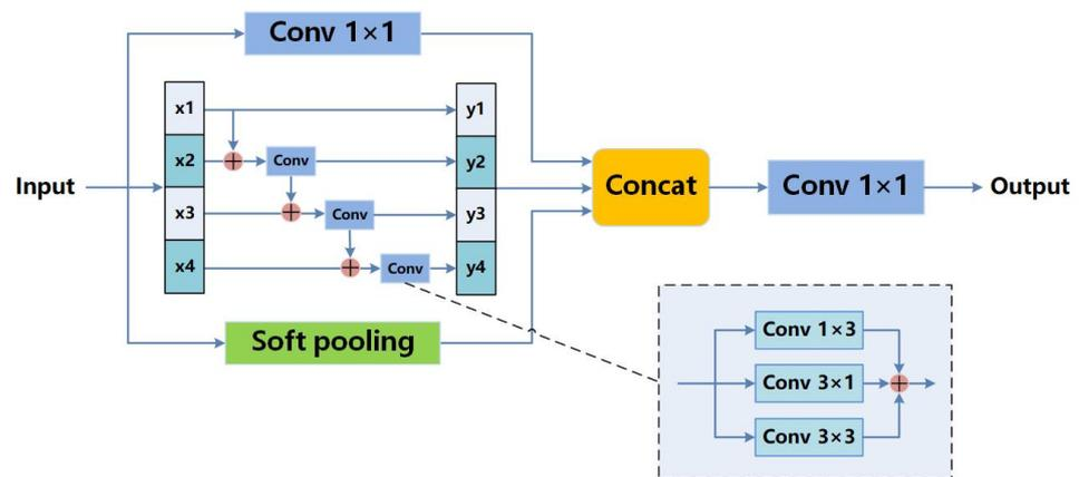
Figure 5. Multi-scale capture block.
