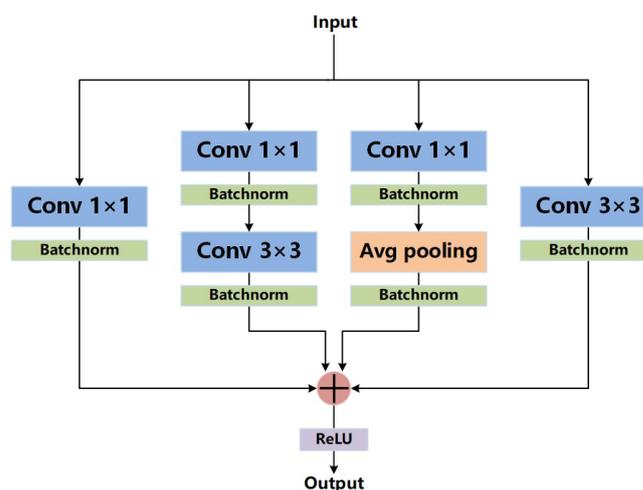
Figure 7. Structure of the diverse branch block.
