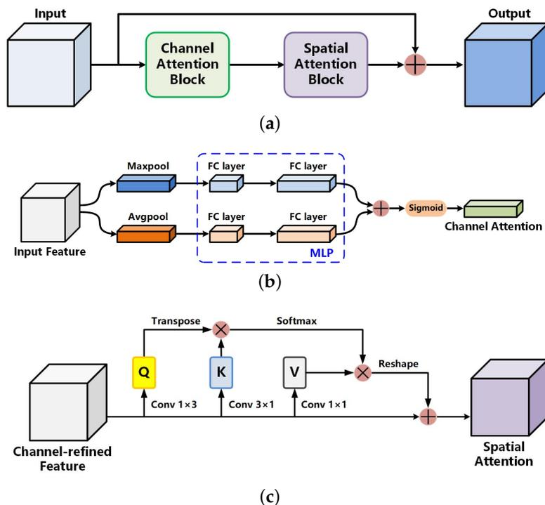
**Figure 4.** Channel and spatial attention block: (a) overall structure; (b) channel attention block; and (c) spatial attention block.
