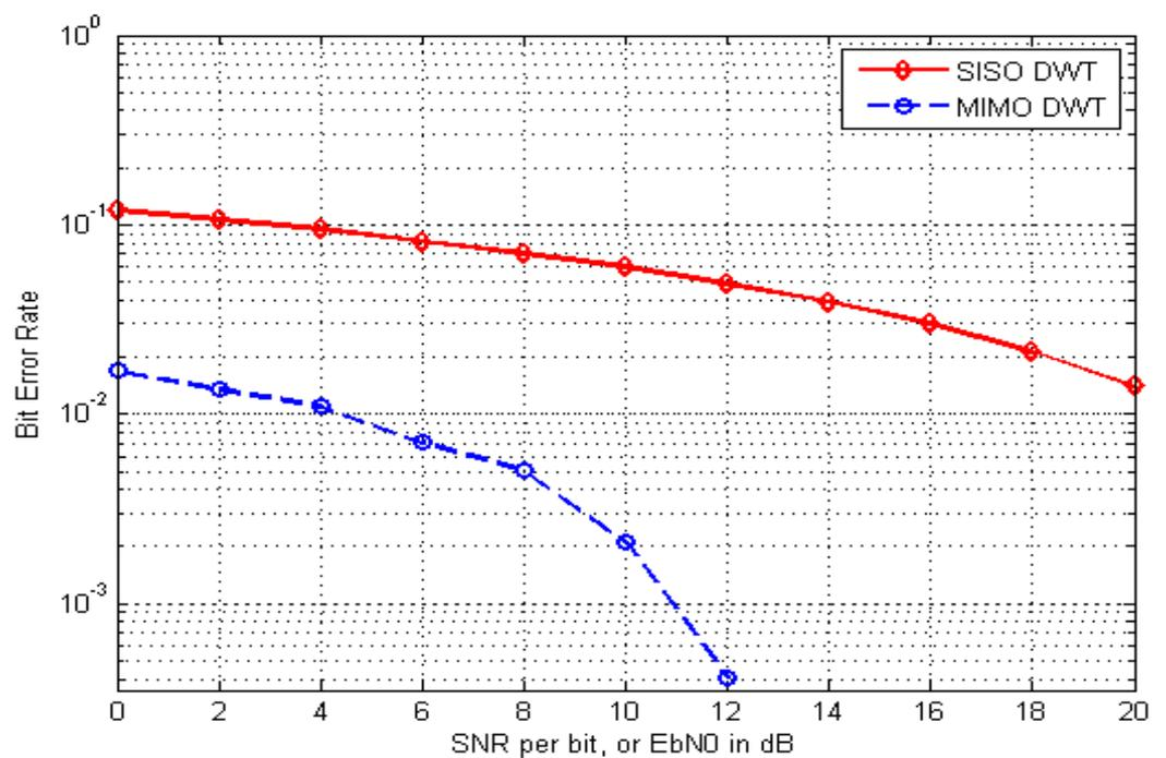
**Figure 4.** MIMO diversity with DWT-OFDM.
