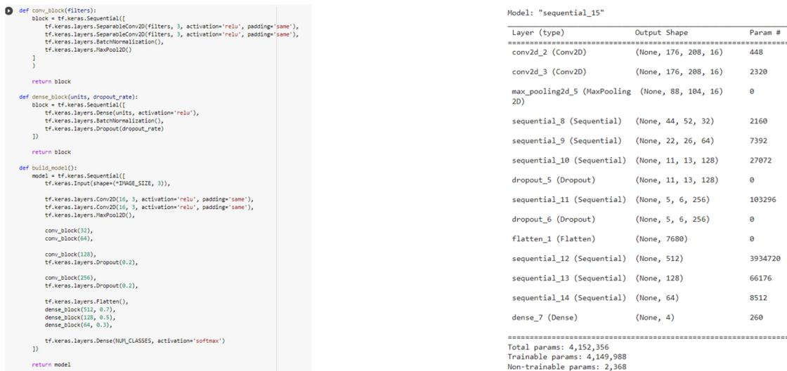
Figure A1. Tensorflow code and model configuration.
