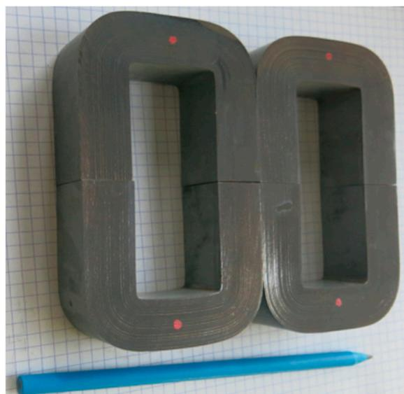
**Figure 4.** Example of wound core made with thin GOES strips insulated by a ceramic coating.
