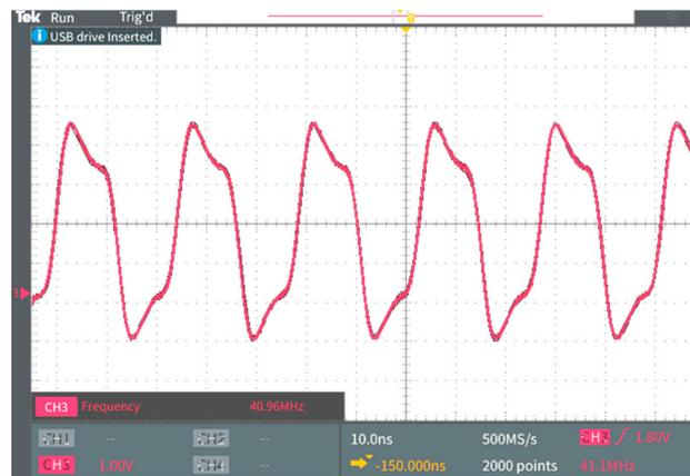
**Figure 11.** Diagram of the output clock.
