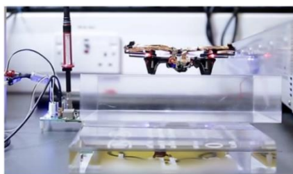
Figure 5. Wireless charging hovering drone. Reproduced with permission from Ref. [22]; published by IEEE, 2017.
