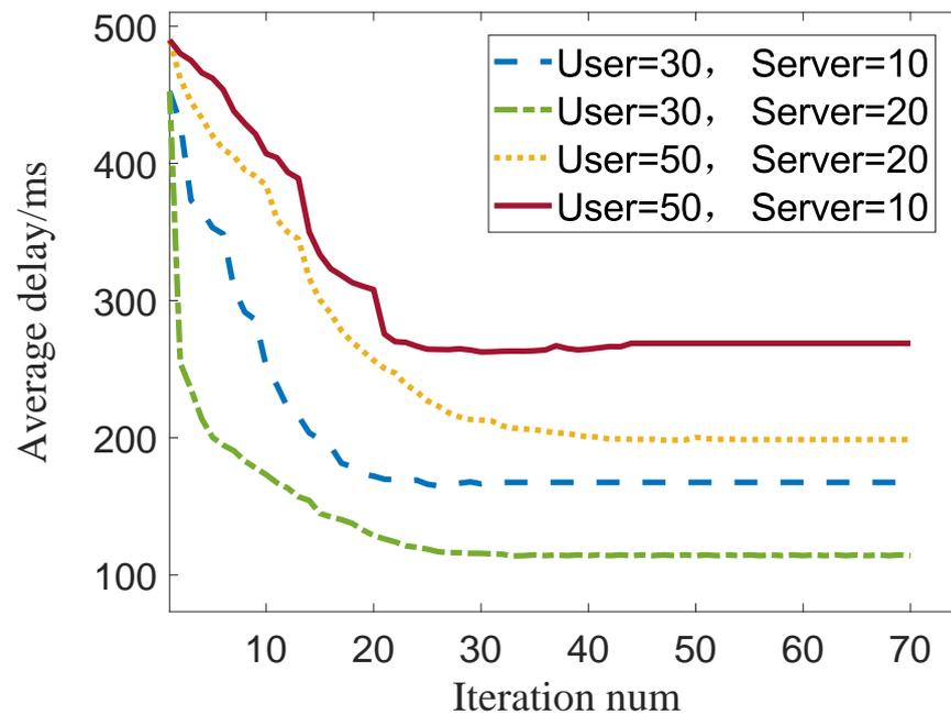
**Figure 3.** The convergence of the distributed DETO algorithm.
