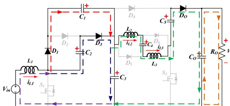
Figure 5. Conduction diagram of the proposed converter in OFF state (Mode 2).
