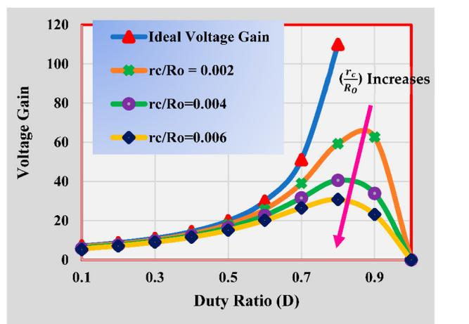
Figure 18. Voltage gain variation as per parasitic resistance of the capacitor.
