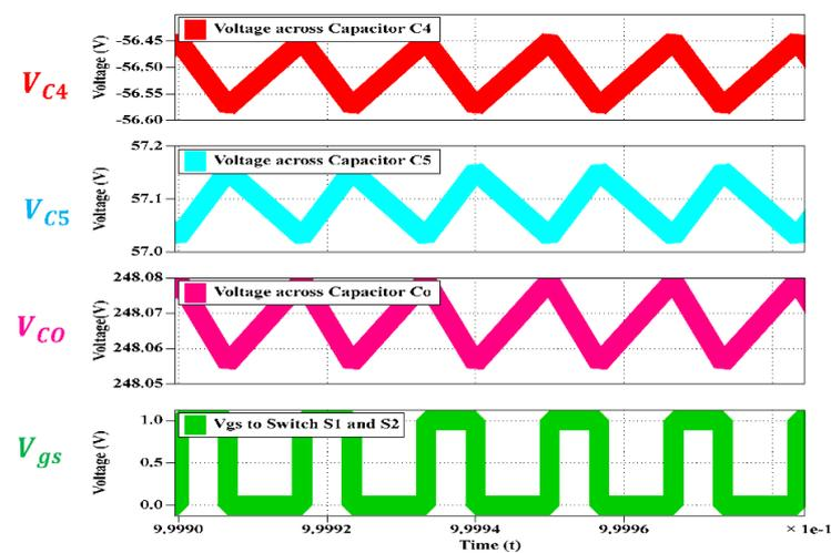
Figure 25. Simulated capacitor voltages and duty cycle (D).
