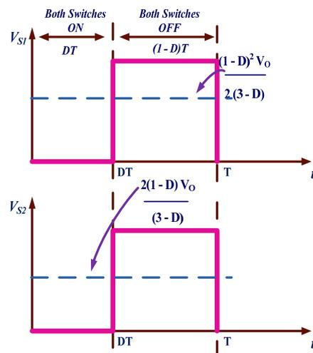
Figure 7. Switch voltages.
