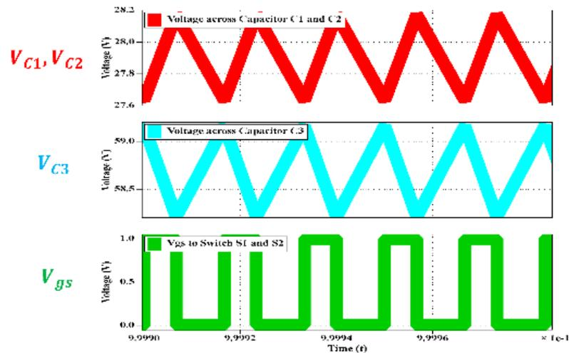
Figure 24. Simulated capacitor voltages and duty cycle (D).
