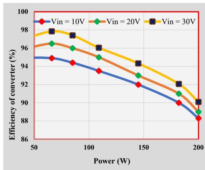
Figure 31. Simulated efficiency vs. output power comparison of the proposed converter at different input voltages.
