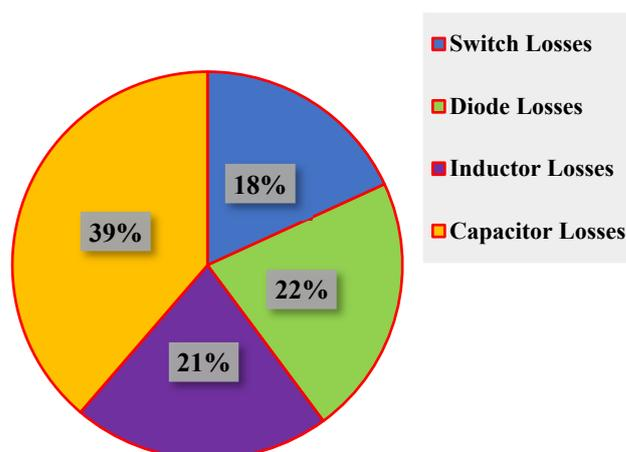
Figure 32. Distribution of losses across various elements of the converter.
