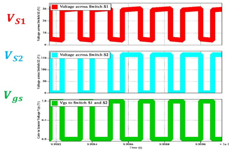
Figure 23. Simulated switch voltages and duty cycle (D).
