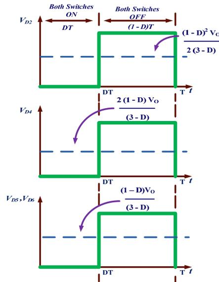
Figure 9. Diode voltages.
