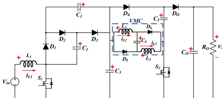
Figure 3. Proposed high-gain dc-dc converter topology.
