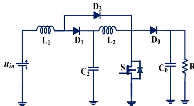
Figure 1. A traditional quadratic boost converter (TQBC).
