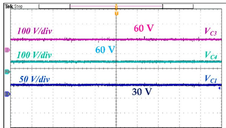
Figure 29. Top to bottom: experimental waveforms of voltage across capacitor  $C_3$  ( $V_{C3}$ ), the voltage across capacitor  $C_4$  ( $V_{C4}$ ), and the voltage across capacitor  $C_1$  ( $V_{C1}$ ) at  $D = 0.4$ .
