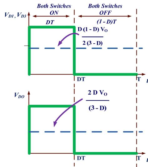
Figure 8. Diode voltages.
